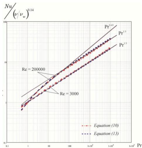
Figure 3: The comparison of Eq.(15) with calculations by Gnielinski (1975) Equation and correlations with fixed  $Pr$  powers.
