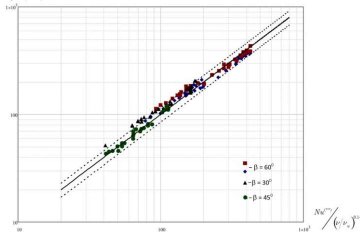
Figure 1: The comparison of  $\text{Nu}^{(*)}$  (solid line) calculated by Eq.(15) with experimental  $\text{Nu}^{(**)}$ : dashed lines corresponds to error  $\pm 15\%$ .
