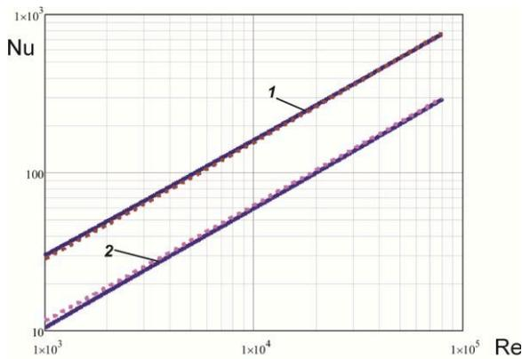
Figure 2: The comparison of  $Nu_{(10)}$  (solid lines) calculated by Eq.(15) with calculated by Eq.(12)  $Nu_{(12)}$  (dashed lines) for  $v/v_w=1$  and  $Pr=1$ : 1 -  $\beta=65^\circ$ ; 2 -  $\beta=30^\circ$ .
