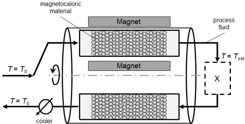
Figure 1: A schematic of active magnetic regenerative heat circulator. X is a process which does not involve exchange of reaction heat.  $T_0$  and  $T_{set}$  denote the environmental temperature and the set temperature at process X respectively
