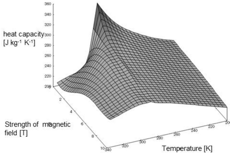
Figure 2: Heat capacity of Gadolinium in the vicinity of its Curie temperature under various magnetic fields
