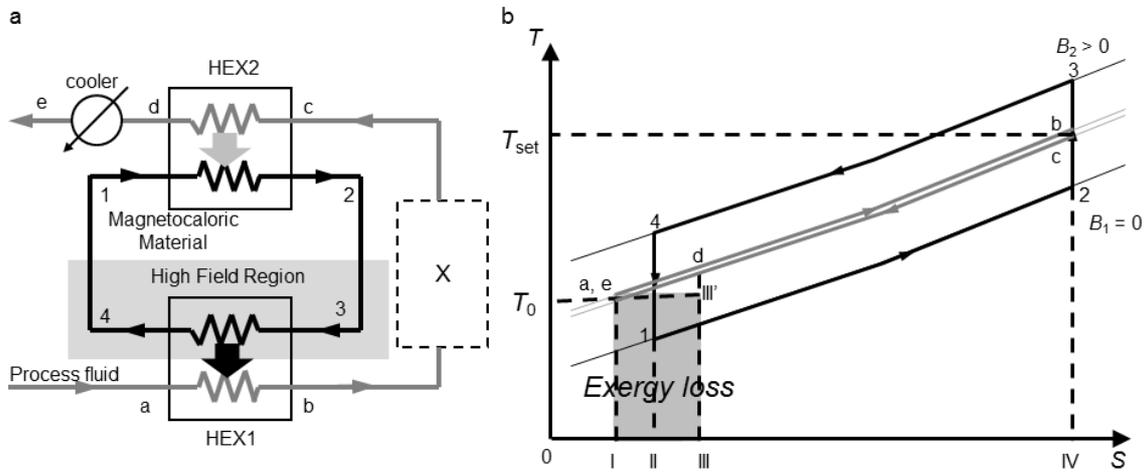
Figure 4: A schematic of heat circulator where magnetocaloric effect is applied, a) process image b) cycle in terms of temperature-entropy diagram
