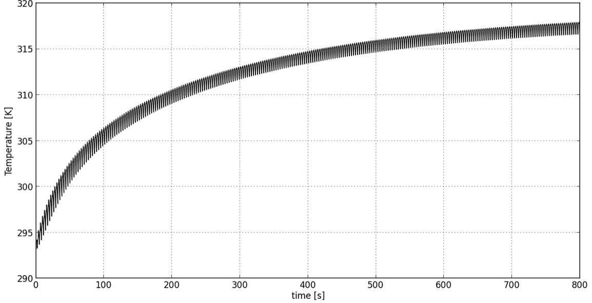
Figure 3: Temperature evolution of the process fluid at the hot end of the active regenerative bed
