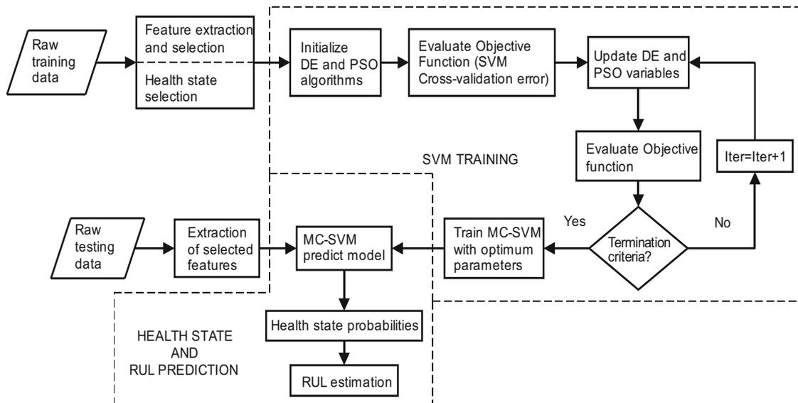
Figure 1: Workflow of the proposed machinery prognostics method
