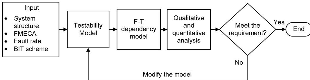
Figure 1: Iterative process of analysis and modification in testability design
