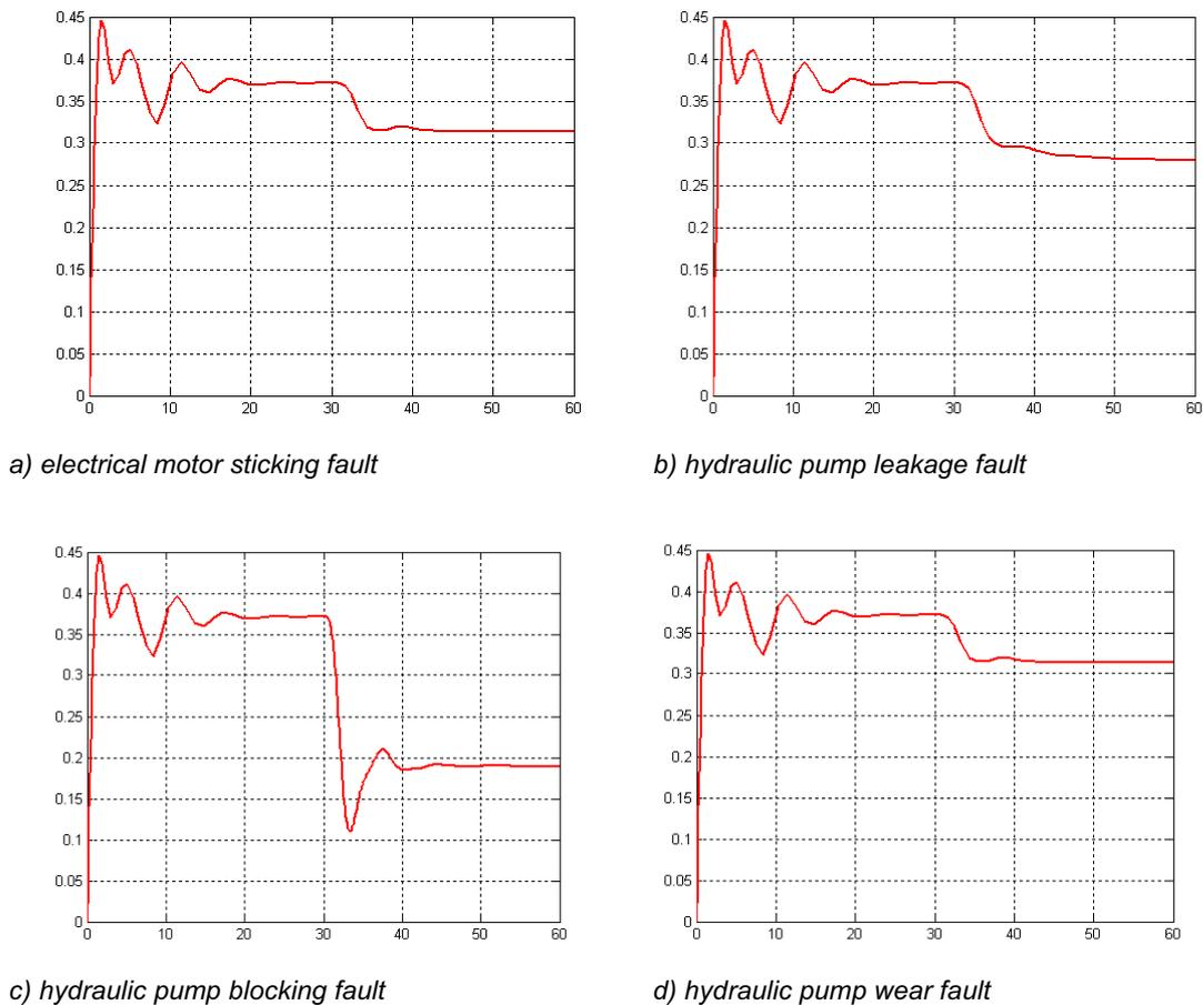
Figure 5: Simulation of angular velocity output of Aircraft rudder
