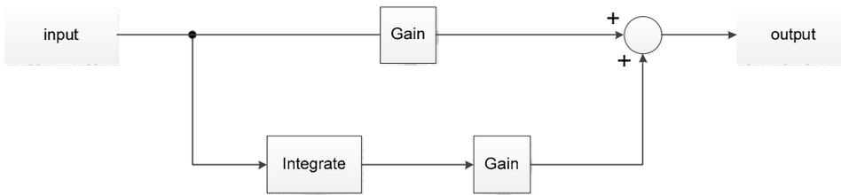
Figure 2: Functional modeling at the subsystem level - Controller
