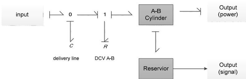
Figure 3: Functional modeling at the subsystem level - Hydraulic cylinder
