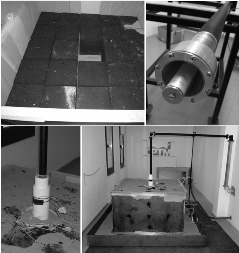
Figure 1: Experimental set up. Oil sands blocks placed in the steel containment tank (top-left); rigid coaxial line terminating in the dipolar antenna (top-right); close up image of the antenna inserted in the low-loss shell (bottom-left); comprehensive view of the set up (bottom-right).
