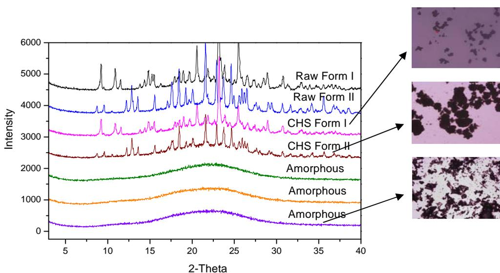
Figure 6. XRD and optical microscopy analysis for; Form II crystallization, Form I and amorphous transformations.
