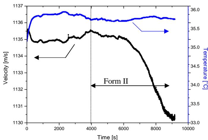
Figure 3.: Ultrasonic velocity profile of FA/IPA in the crystallization of CHS Form II
