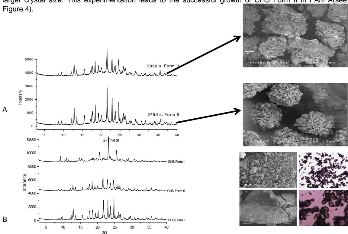
Figure 4. PXRD, SEM, optical microscopic image of CHS Form II; (A) 0.05 gFA/gIPA; (B) 0.5 gFA/gIPA
