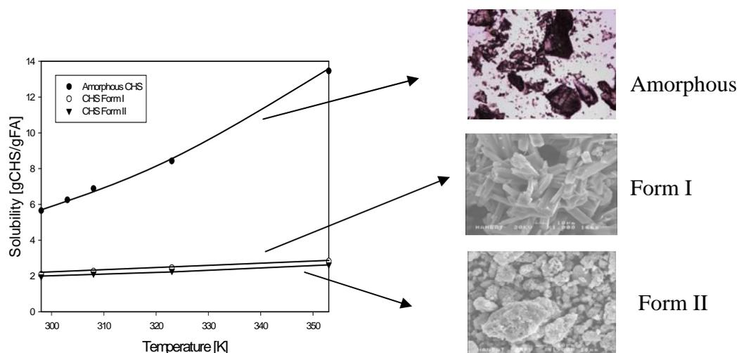
Figure 2: Solubility of amorphous, Form I and II in formic acid at different temperatures
