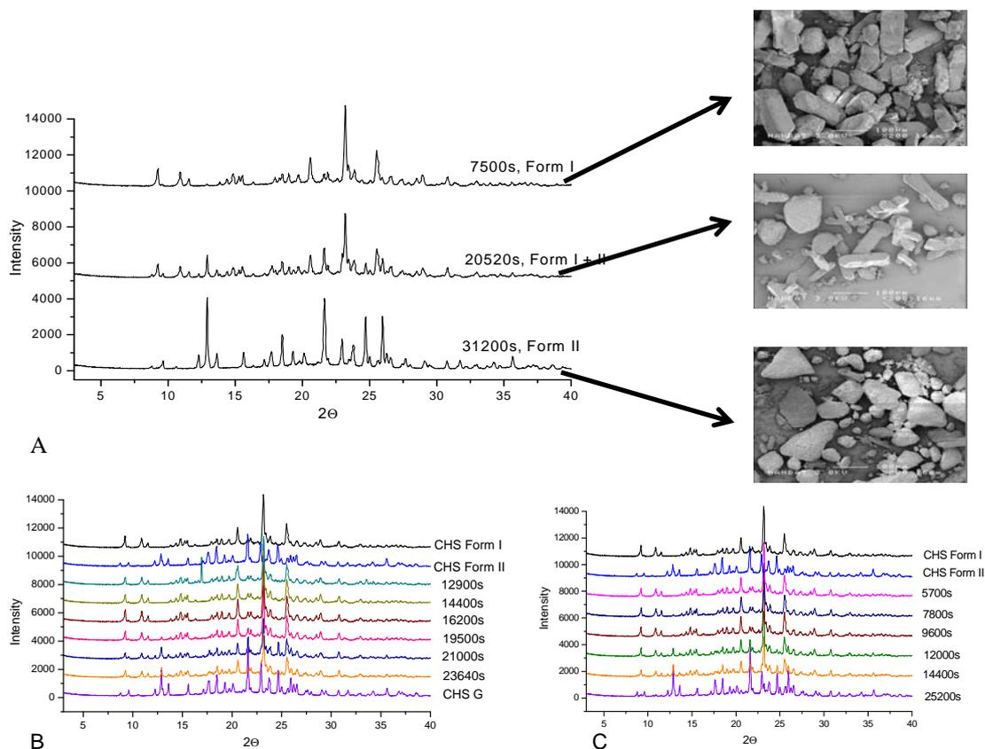
Figure 5: Transformation of CHS Form II; (A) PXRD and SEM analysis, (B) PXRD analysis, (C) PXRD analysis
