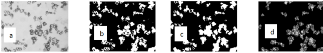
Figure 2: (a) Original, (b) Edge detection binary image, (c) Crystal clusters binary image, (d) Crystal clusters image.
