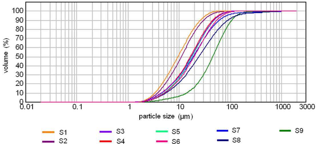
Figure 3: Particle size distribution results of sediment samples (Malvern 2000, UK)
