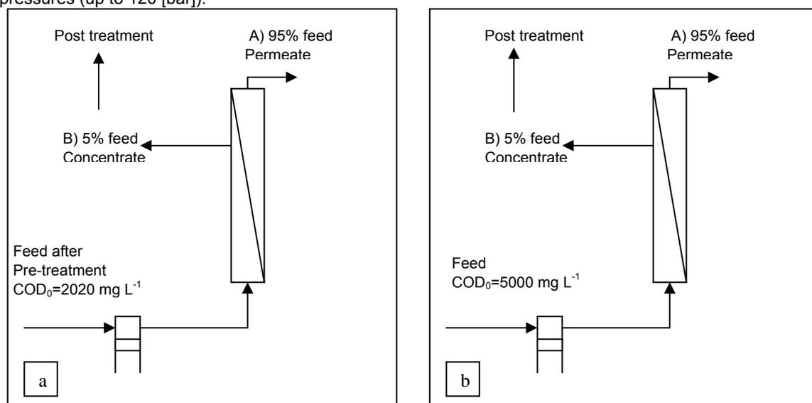
Figure 4: Flow sheet of two different configuration
