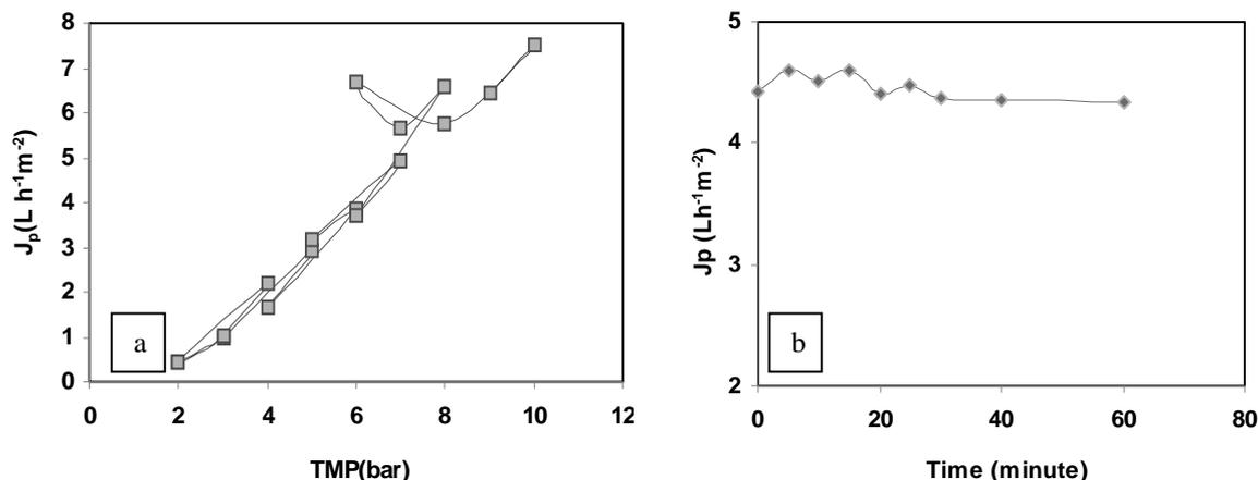
Figure 2:a) Threshold flux determination of tannery waste water using NF module b) Permeate flux profile operating condition 6 bar
