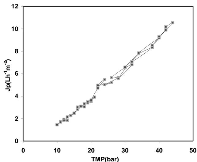
Figure 3: Threshold flux determination of tannery waste water using RO
