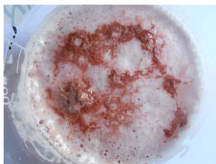
Figure 2: Picture of agglomerates formed in the aphron phase recovered from the separation trials carried out with undiluted extract.
