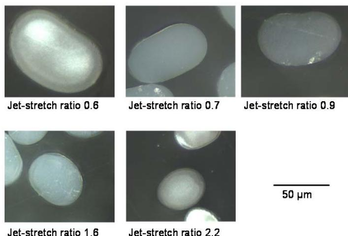
Figure 5: Light microscopy images of air-gap spun fibres with different jet-stretch ratios
