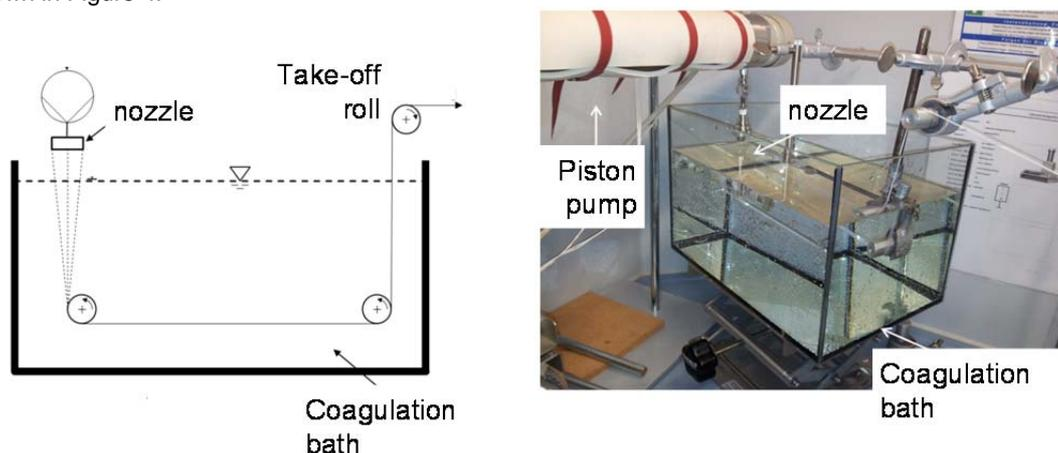
Figure 4: Experimental setup: Scheme (left) and photography (right)
