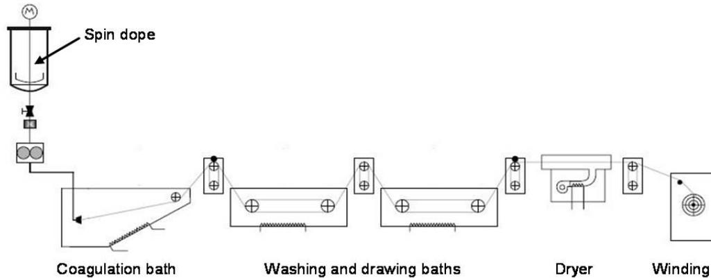
Figure 1: Wet spinning process for the production of carbon fibre precursors
