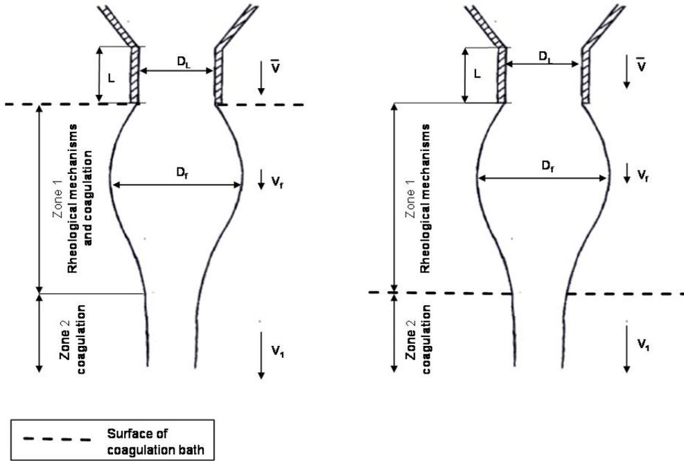
Figure 2: Fluid dynamics in the nozzle and in the forming fibre for wet-spinning (left) and air-gap spinning (right) partly based on (Falkai, 1981)
