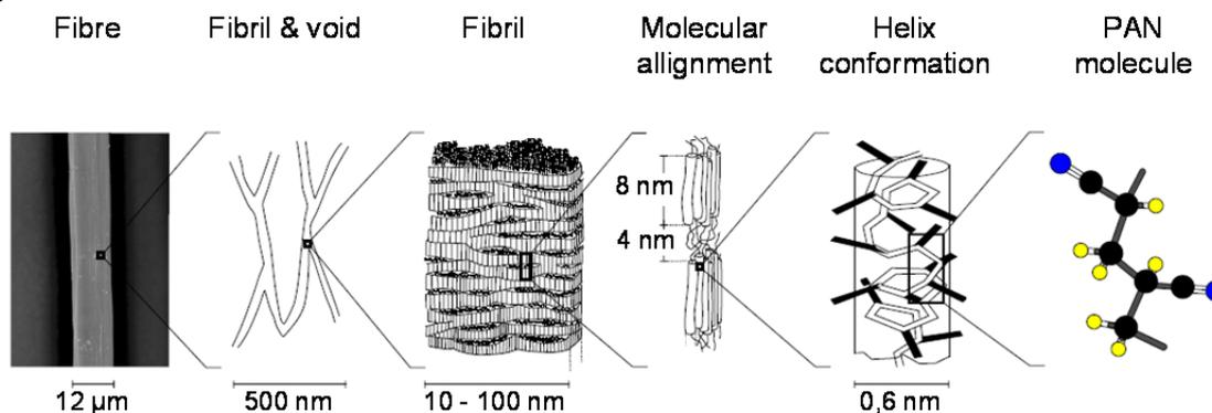
Figure 3: Fibre structure of a PAN precursor, partially based on (Masson, 1995)
