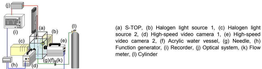
Figure 6. Experimental setup for the single bubble measurement.
