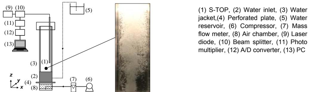
Figure 5. Setup for the bubble column measurement (the image is captured by SONY digital handy-cam).
