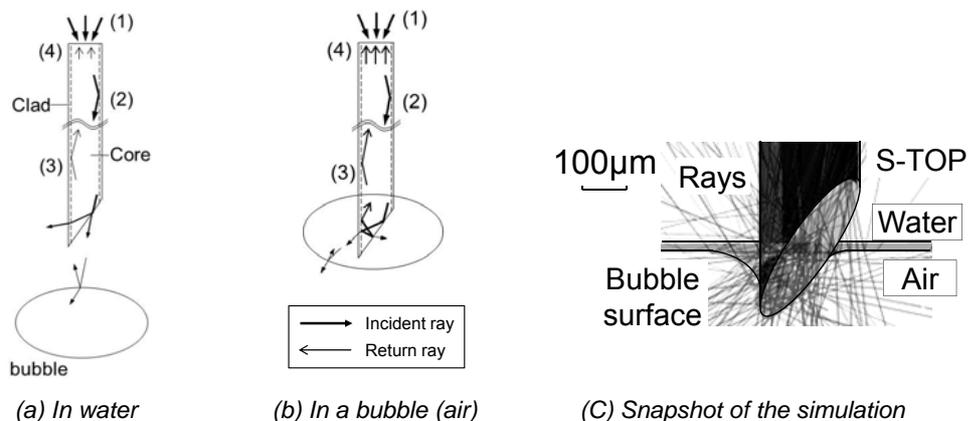
Figure 4. Schematic of the numerical simulation. (1) The rays are introduced. (2) The rays iterate total reflection. (3) Depending on the conditions, rays return. (4) The returned rays' energy is sum up.
