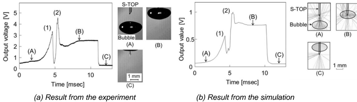
Figure 8. Typical experimental result and numerical result of the S-TOP.
