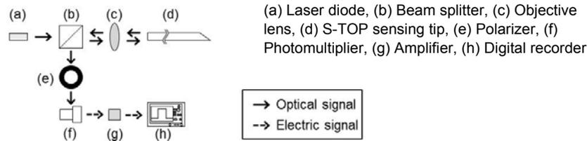
Figure 1: Optical system of the S-TOP measurement.
