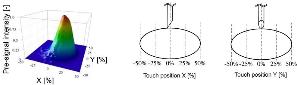
Figure 10. 3D simulated result of relationship between the pre-signal intensity and touch positions.
