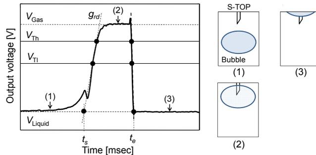
Figure 3. Typical output signal of the S-TOP in the bubble measurement.
