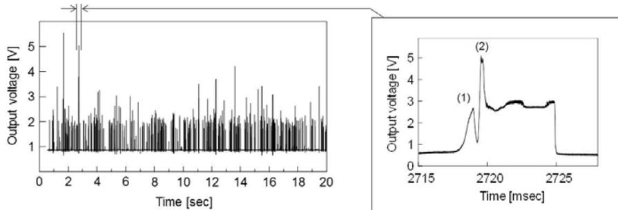
Figure 7. Time series output signal from the S-TOP in the bubbly flow. A typical burst signal is extracted.
