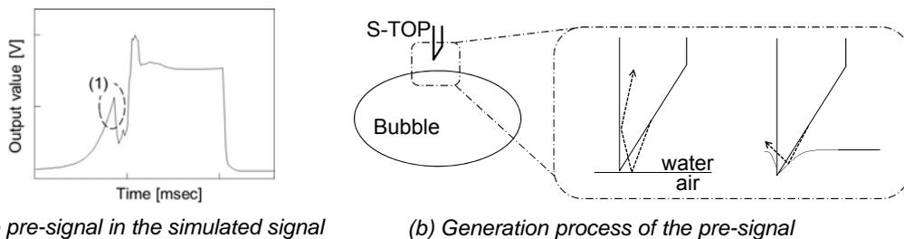
(a) The pre-signal in the simulated signal (b) Generation process of the pre-signal
