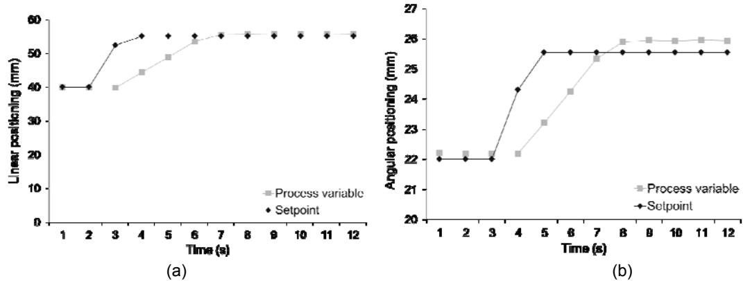
Figure 3: Profile of a) linear and b) angular motion displacement of the process variable relative to the setpoint in relation to the time when the reset automatic mode was tested.
