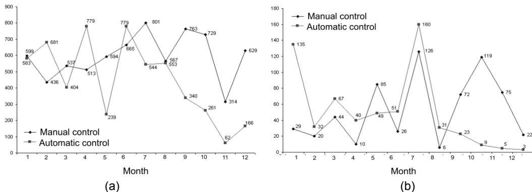
Figure 4: Number of occurrences of scrap (weight) before and after the implementation of the control system a) of PGZN and b) of PBOR.
