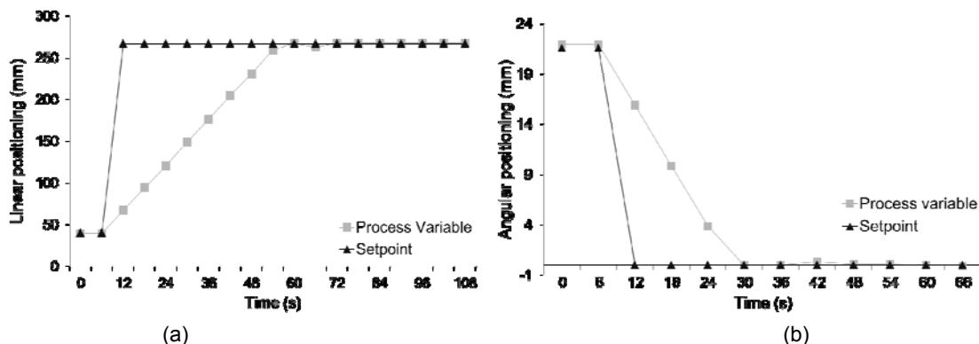
Figure 2: Profile of a) linear and b) angular motion displacement of the process variable relative to the setpoint in relation to the time when the reset automatic mode was tested.
