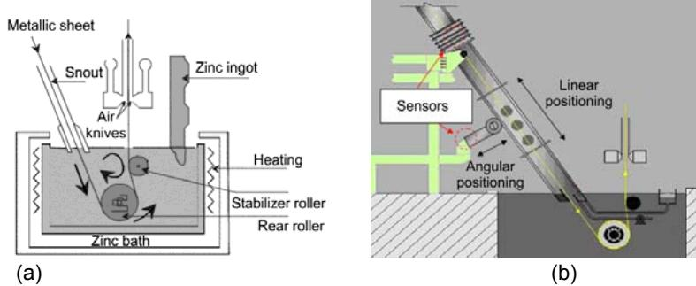
Figure 1: a) Schematic diagram of the zinc bath of galvanization process and b) illustration of the installation of the linear and angular positioning sensors used for position determination.
