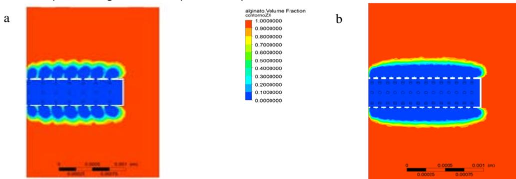
Figure 4: Flow of water into alginate in one single needle: (a) with 7 rings, (b) with 14 rings (more homogeneous spreading).
