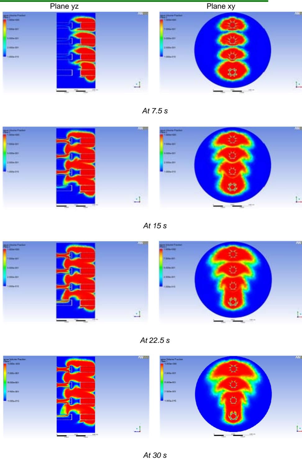
Figure 5: Water volume for outlet velocity equals to 5 mm/s at different moments.
