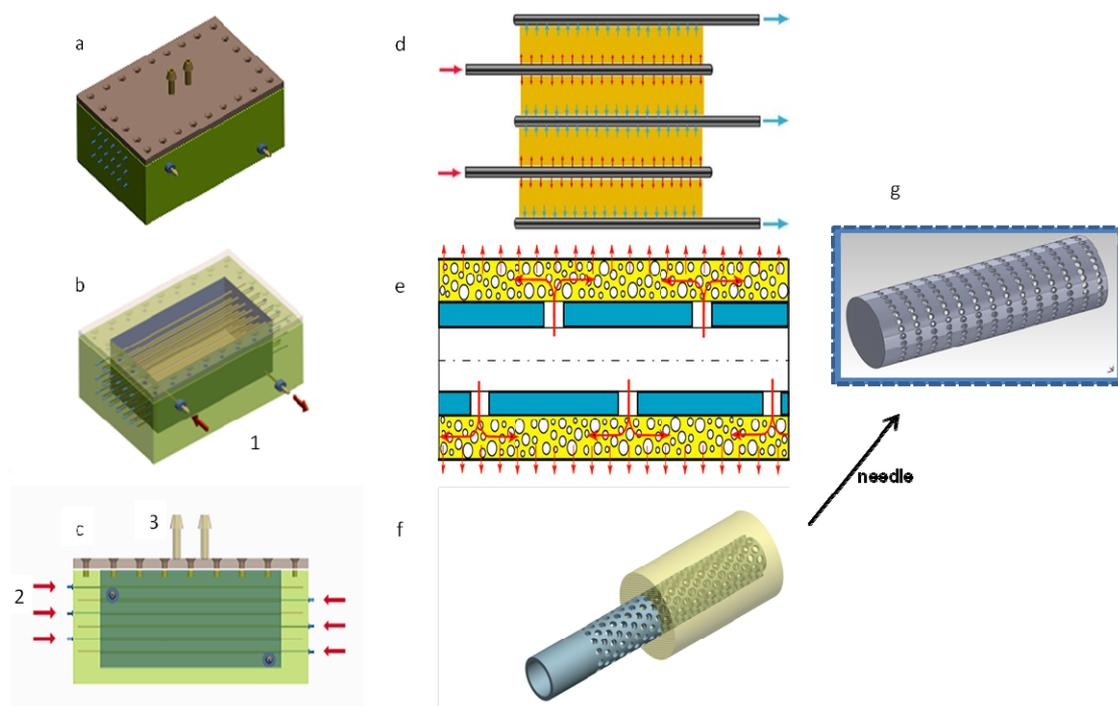
Figure 2. Design of an irrigating triple perfusion bioreactor.
