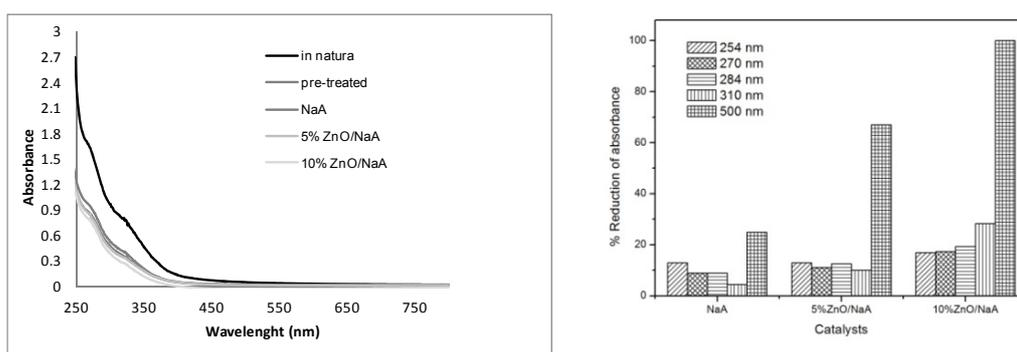
Figure 6: UV-Vis spectra and reduction of absorbance: vinasse in natura, pre-treated and photocatalysis.
