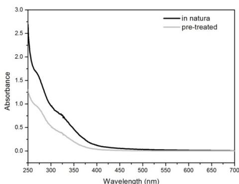
Figure 1: UV-Vis spectra of vinasse *in natura* and pre-treated with Tanfloc<sup>®</sup>.
