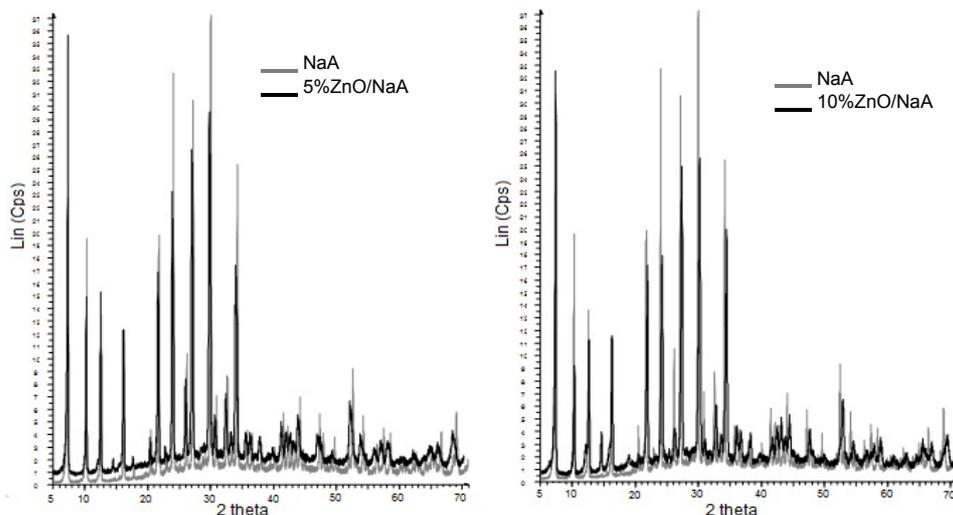
Figure 2: Diffractograms of pure zeolite NaA and supported catalyst.
