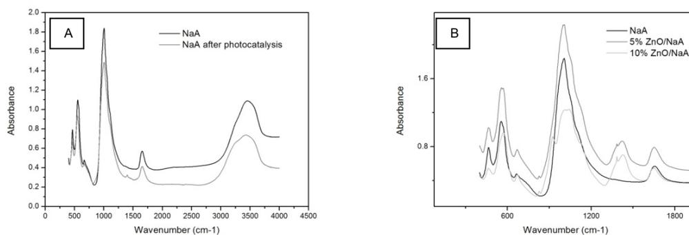
Figure 3: Infrared spectra of pure zeolite (A) and supported catalysts (B).
