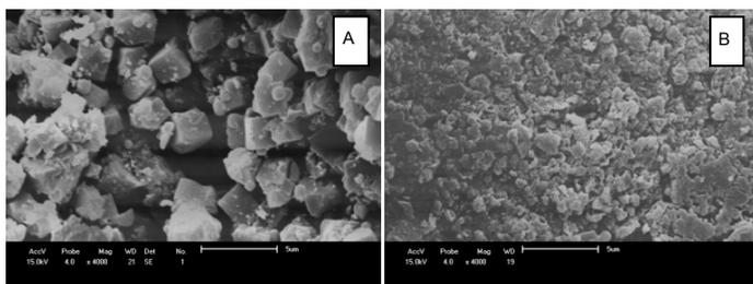
Figure 4: Micrograph of pure zeolite NaA (magnification 4000x).
