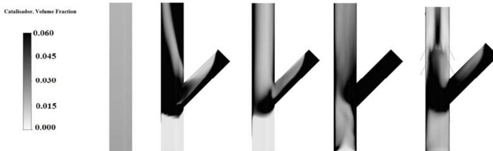
Figure 5. Field of the solids holdup for cases 1-5
