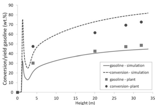
Figure 4. Predicted model results and the plant data reported by Derouin et al. (1997) along the riser center line.
