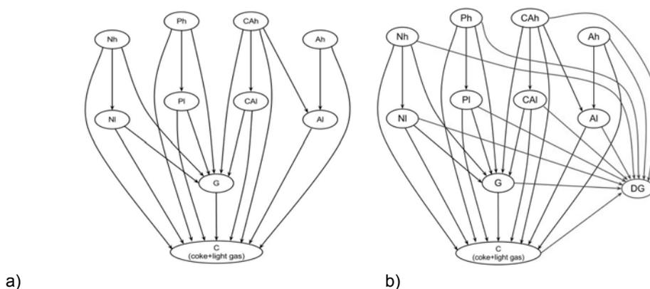
Figure 3. a) 10-lump kinetic model proposed by Jacob et al. (1976) b) Adapted kinetic model (11-lumps)
