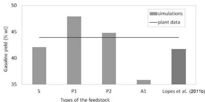
Figure 5: Gasoline yields at the riser outlet
