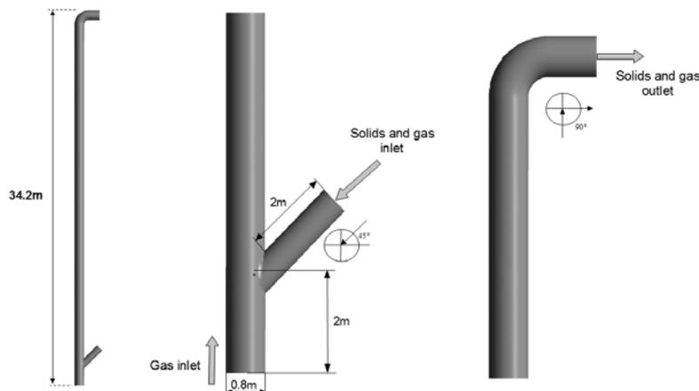
**Figure 1.** Geometry of the riser Lopes et al. (2011a)
