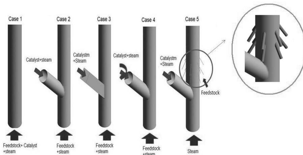
Figure 2. Configurations proposed to feed the catalyst particles
