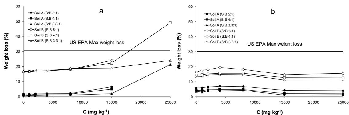
Figure 4: Effect of Pb soil concentration on the weight loss of S/S treated soils during freeze-thaw (a) and wet-dry (b) durability test for soil A and B (S:B ratio of 3.3, 4.0 and 5.0)
