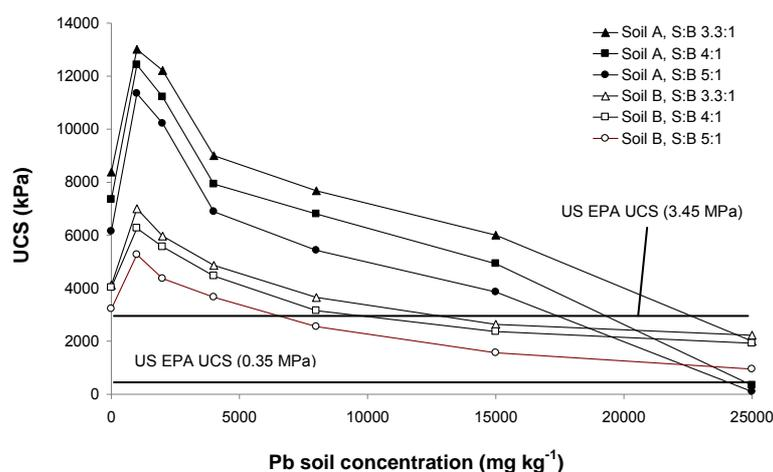
Figure 2: Effect of Pb soil concentration on the UCS development of S/S soils for soil A and B (S:B ratio of 3.3, 4.0 and 5.0)
