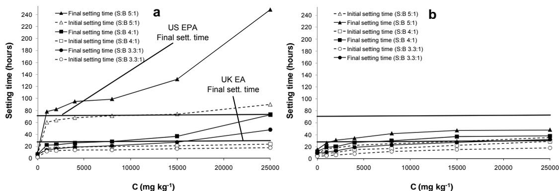
Figure 1: Setting times of S/S treated soils vs Pb soil concentration (C) for soil A (a) and soil B (b) (S:B ratio of 3.3, 4.0 and 5.0)
