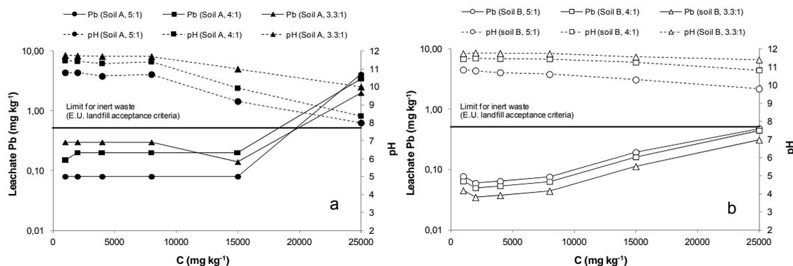
Figure 3: Effect of Pb concentration on the leachability of Pb and pH of S/S soils for soil A (a) and B (b)
