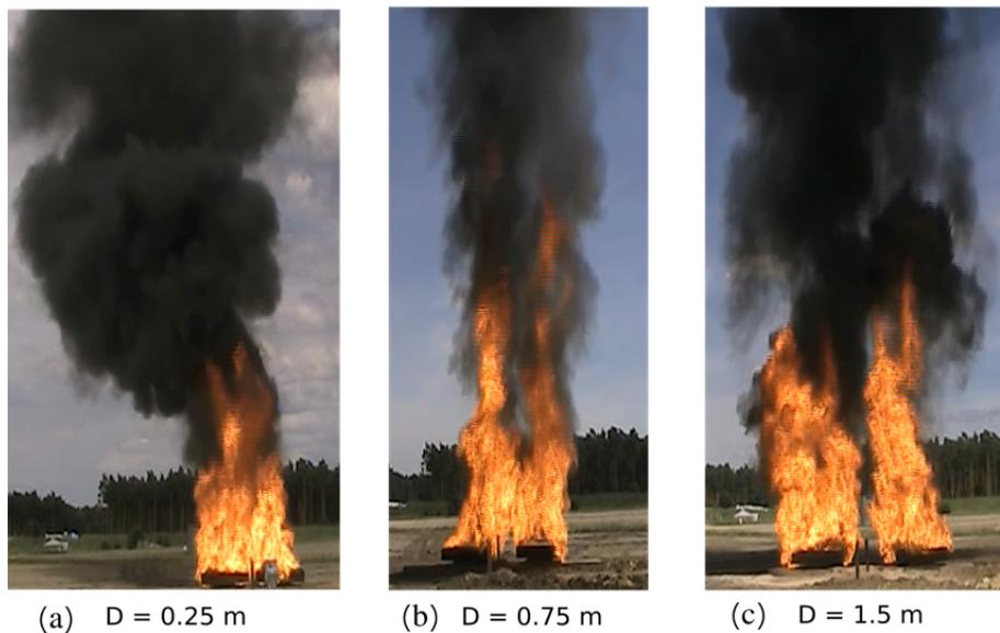
Figure 2: Flame merging of multiple hydrocarbon pool fires in laboratory scale and field experiment
