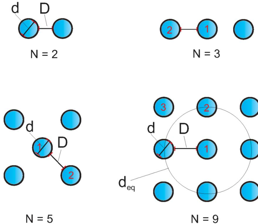
Figure 1: Experimental arrangements for the investigation of multiple fires
