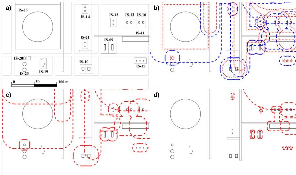
Figure 2: Layout considered in the case-study and footprint of the fireproofing zones according to the criteria of Table 1. Panel a) layout and location of isolable sections. Panel b) fireproofing zones for structural elements; red (internal) area: impingement zone (S1); blue (outer) area: radiative heat zone (S2). Panel c) fireproofing zone for atmospheric vessel targets (AV). Panel d) fireproofing zone for pressurized vessel targets (PV).
