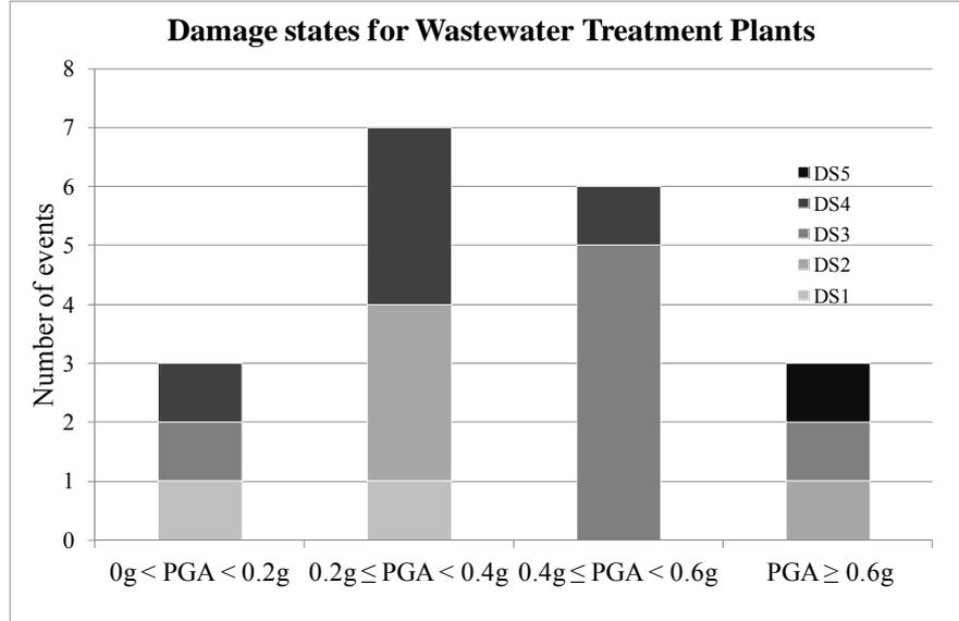
Figure 1: Number of events of damage states DS for WWTPs.
