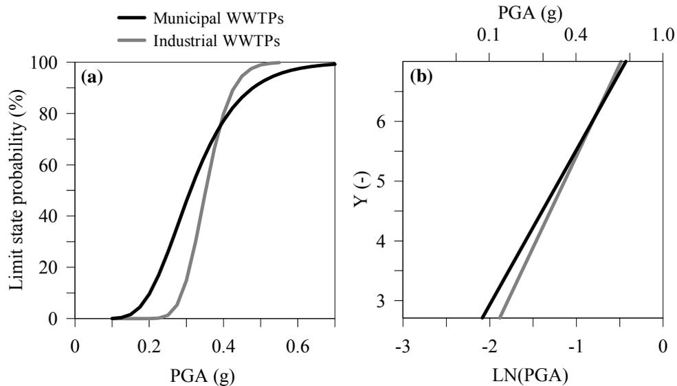
Figure 2: Fragility (a) and probit (b) curves for WWTPs.
