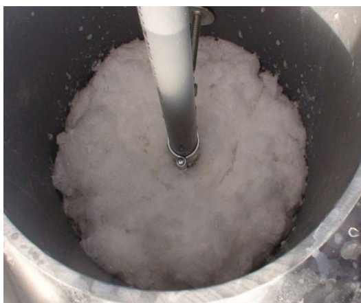
Figure 2: Foam at the upper part of reactor
