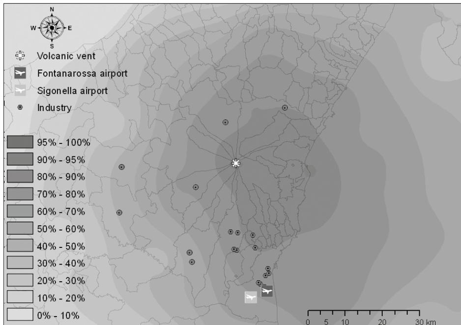
Figure 3: Vulnerability map for light damage of fixed roof storage tanks using the deterministic approach of Inverse Distance Weighting.
