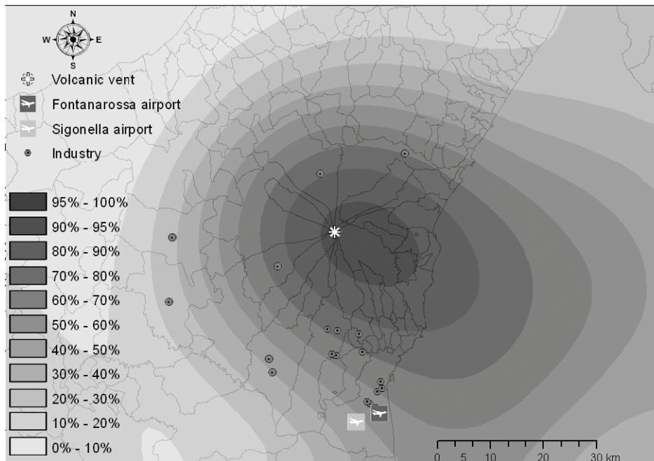
Figure 4: Vulnerability map for light damage of fixed roof storage tanks using the geostatistical approach of Kriging.
