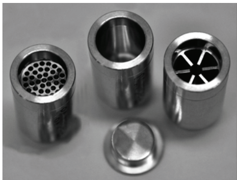
Figure 4: Sample cells for the SETARAM C80 twin calorimeter: In the middle: conventional "beaker type" sample cell. Right: cell with six heat exchange fins- Left: cell 37 micro tubes.
