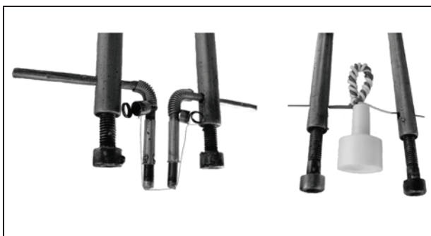
Figure 1: Exploding wire with electrodes (left side) and pyrotechnical igniter (right side)
