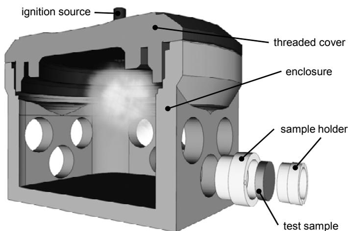
Figure 1: Experimental setup in principle showing enclosure 1 as an example, including one sample holder and a test sample
