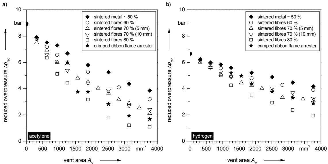
Figure 2: Reduced explosion overpressure  $\Delta p_{red}$  within enclosure 1 as a function of vent area  $A_v$  using different porous structures; a)  $(14 \pm 1)$  vol. % acetylene/air mixture and b)  $(31 \pm 1)$  vol. % hydrogen/air mixture
