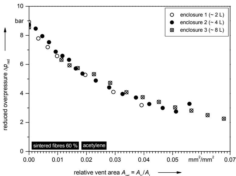
Figure 3: Reduced explosion overpressure  $\Delta p_{red}$  as a function of relative vent area  $A_{rel}$  within three different enclosures using sintered fibre structures with a porosity of 60 %, using a  $(14 \pm 1)$  vol. % acetylene/air mixture
