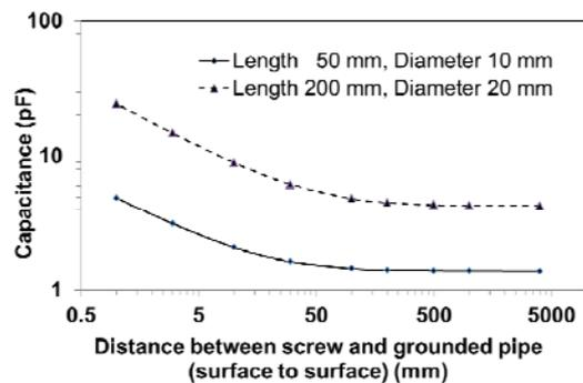
Figure 8: Capacitance of screws close to a grounded metal pipe of diameter 200 mm, length 3.8 m mounted parallel to screw axis.
