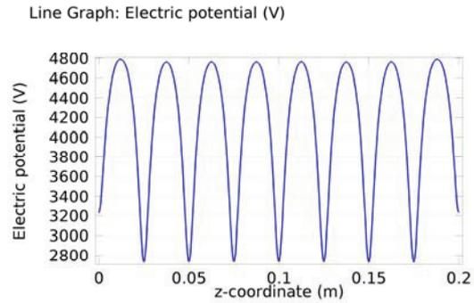
Figure 13: Surface potential at the inner wall in axial direction. With an earthed conductive layer on the outside.
