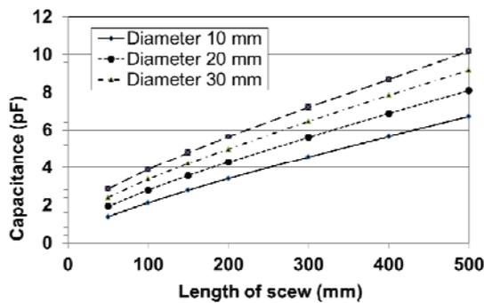
Figure 7: Capacitance of screws in free space.
