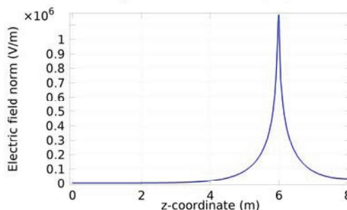
Figure 4: Field strength at the inner silo wall along the z-axis (silo height) with allowing for charge relaxation  $\rho = 5 \cdot 10^{12} \Omega \cdot m$ .
