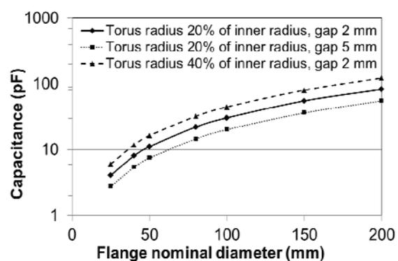
Figure 10: Capacitance of flange (torus) mounted on a grounded metal pipe without making contact (gap width of 2 mm and 5 mm respectively).
