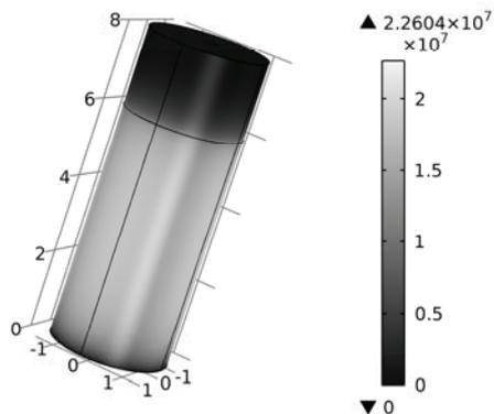
Figure 1: Field strength at the inner silo wall without allowing for charge relaxation.
