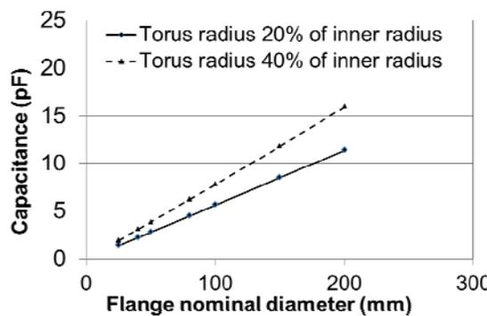
Figure 9: Capacitance of flange (torus) in free space.
