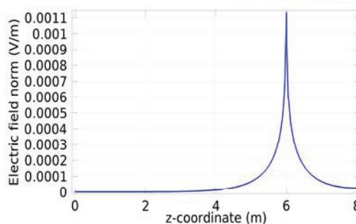
Figure 6: Field strength at the inner silo wall along the z-axis (silo height) with allowing for charge relaxation  $\rho = 5 \cdot 10^{10} \Omega \cdot m$ .
