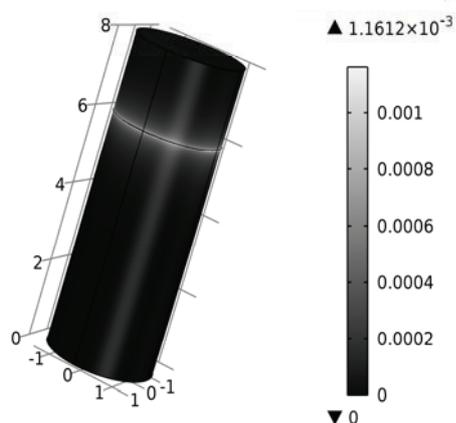
Figure 5: Field strength at the inner silo wall with allowing for charge relaxation  $\rho = 5 \cdot 10^{10} \Omega \cdot m$ .
