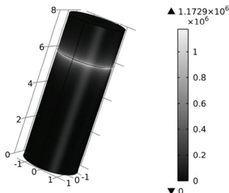
Figure 3: Field strength at the inner silo wall with allowing for charge relaxation  $\rho = 5 \cdot 10^{12} \Omega \cdot m$ .
