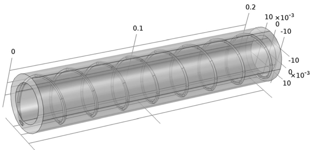
Figure 11: Geometry of the hose used for the model calculations
