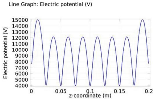
Figure 12: Surface potential at the inner wall in axial direction. Without a conductive layer on the outside.
