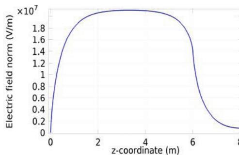
Figure 2: Field strength at the inner silo wall along the z-axis (silo height) without allowing for charge relaxation.
