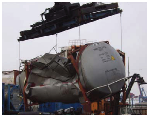
Figure 3: Tank deformed by vacuum damage
