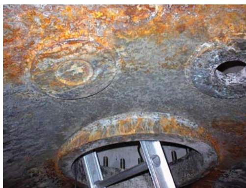
Figure 2: Corrosion in a tank container made of austenitic CrNiMo-steel (1.4571) after transport of sulphur dichloride
