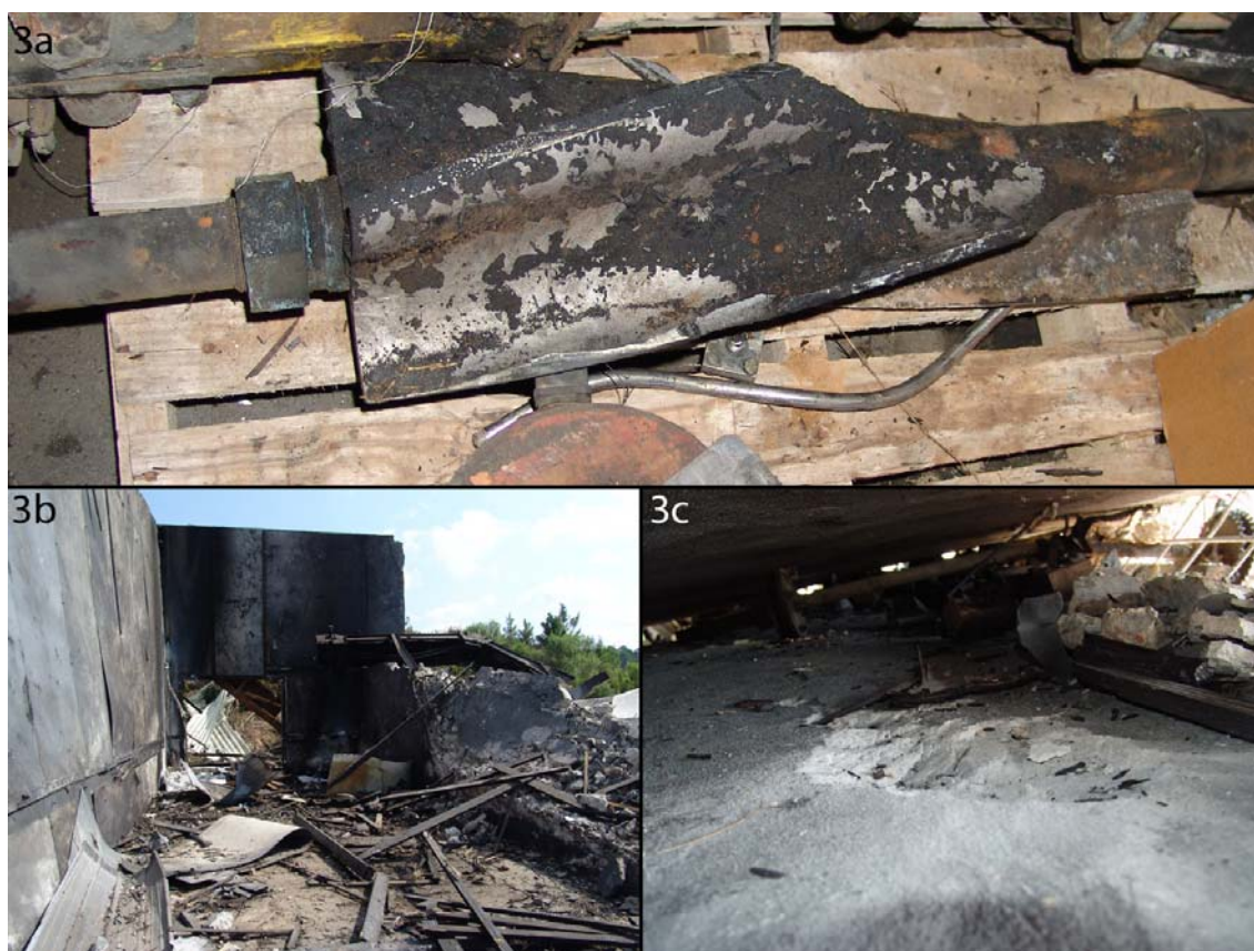
Figure 3: Fragmented worm (a), destroyed corning mill (b) and crater under hopper and worm (c)
