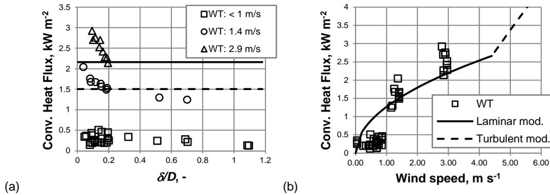
Figure 3: Validation of modelling (solid and dotted lines) with experimentally determined convective heat flux to the pool: (a) The bund walls height effect; (b) wind speed effect
