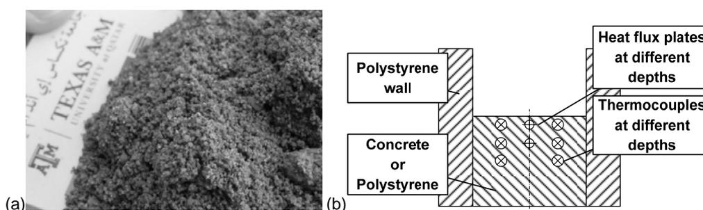
Figure 1. The picture of the concrete powder (a) and the general scheme of the experimental pad (b)
