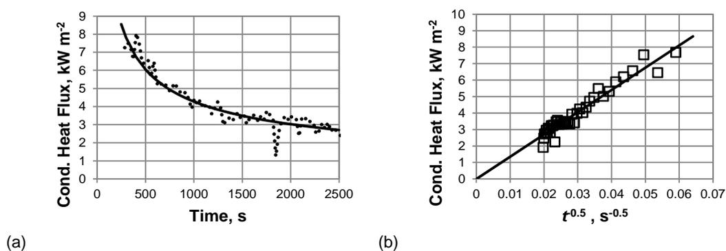
Figure 2. Experimental data of conduction and model fitting (solid line): (a) timeline; (b) linear behaviour of heat flux to inverted square root of time
