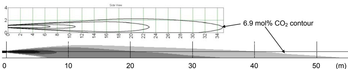
Figure 5: Vertical cross-sections of the Phast (top) and CFD (bottom) CO<sub>2</sub> plumes for a 1-inch (25.4 mm) diameter orifice. Contours of concentration are shown in each case for 6.9, 10, 20 and 30 mol% CO<sub>2</sub>
