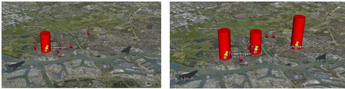
Figure 4: Human perceived odour complaints assigned to e-nose readings (left) and proof-of-principle: All e-noses inside the complaint plot observe the same fingerprint. The others don't (right)
