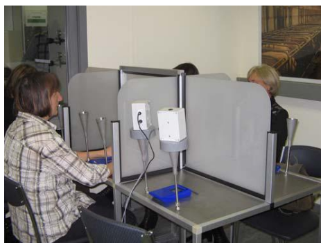
Figure 7: E-nose training with olfactometric analyses: e-nose replace one panellist during an olfactometric test (left), e-nose results for methyl mercaptan (right)
