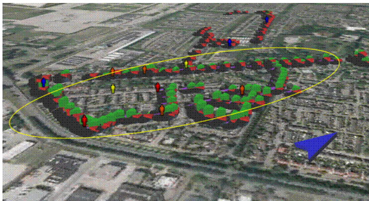
Figure 3: Emission recorded by a mobile e-nose in the residential area. Especially the green sensor reading correlated with human odour observation of burned nuts (red, orange, yellow, blue= intense, moderate, little and no smell).
