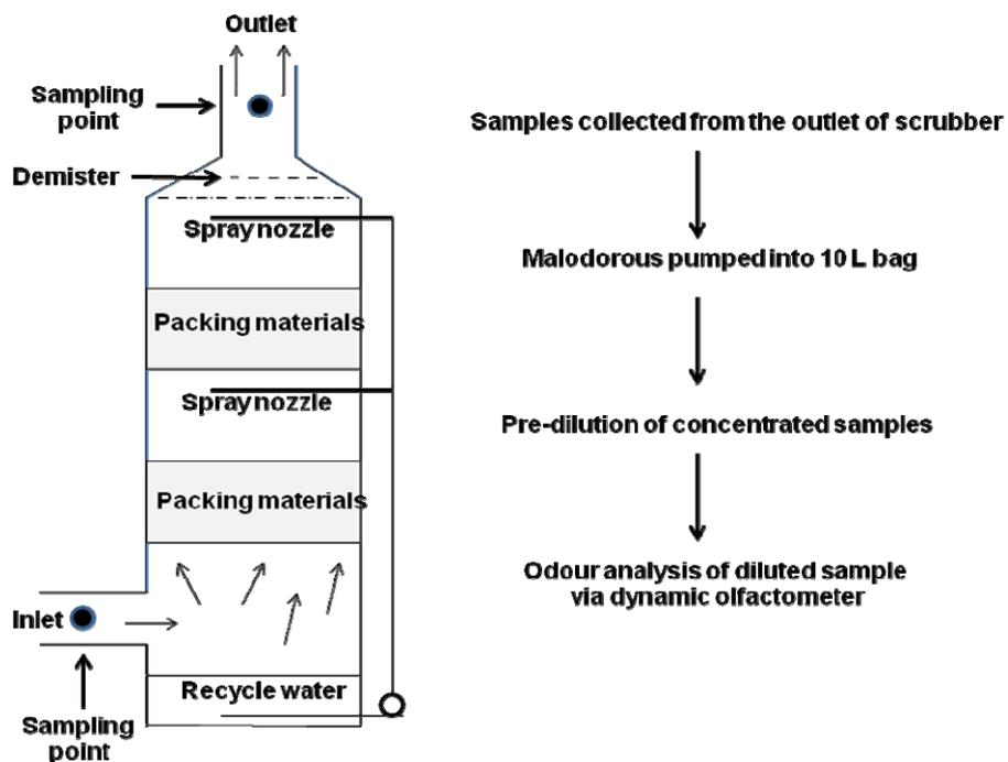
Figure 1: Schematic diagram of a typical water scrubber system and odour sampling methods.
