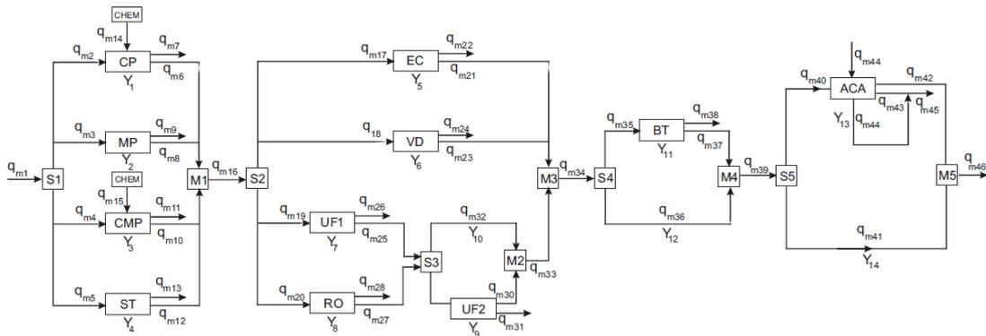
Figure 1: The superstructure of the wastewater separation process.
