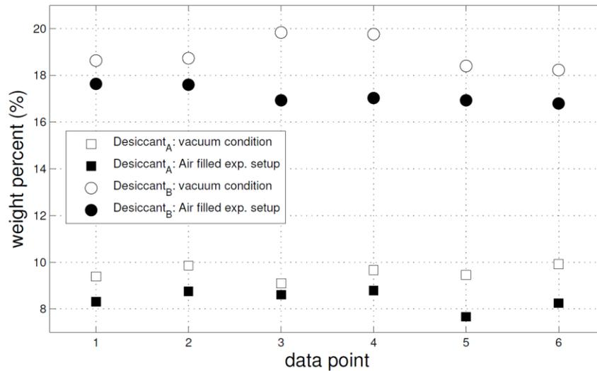
Figure 2: Comparison of the storage capacity in weight percent of desiccant A and desiccant B at 230 °C and with a generated vacuum or air filled in the experimental setup
