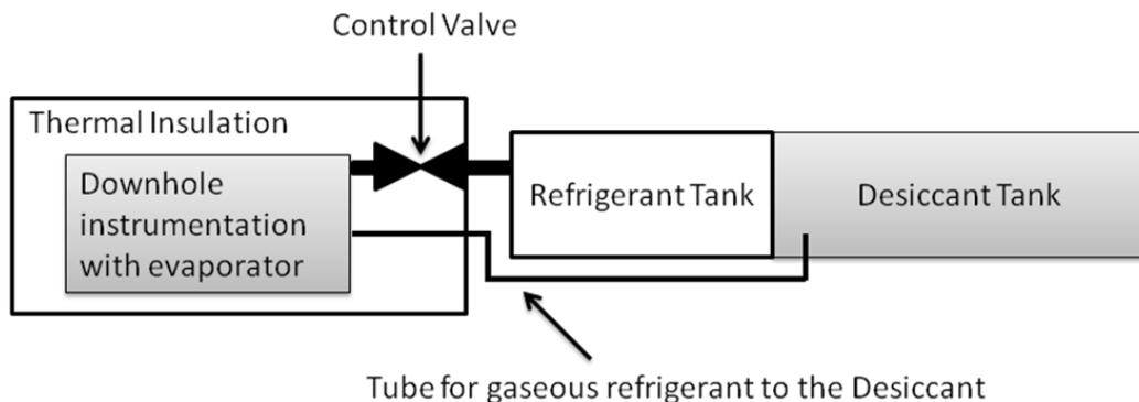
Figure 1: Schematic design of a downhole sorption cooler, thermal insulation, required components and electronics.
