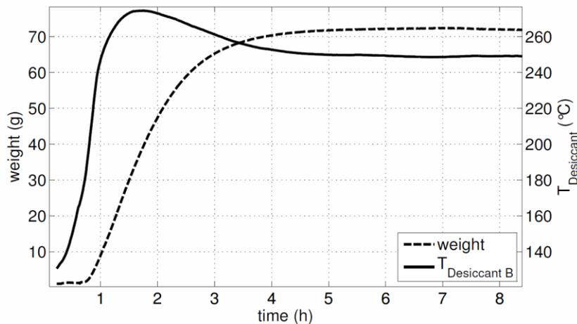
Figure 4: Weight of stored refrigerant and temperature of desiccant B with vacuum condition in the experimental system.
