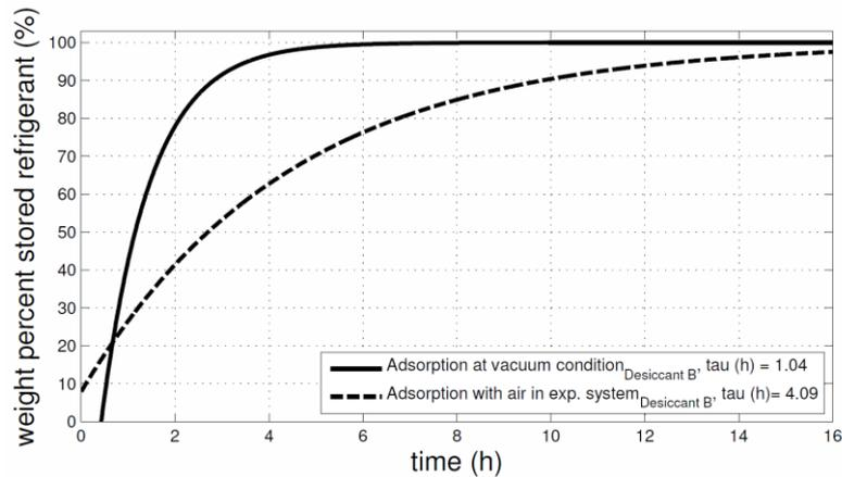
Figure 5: Weight percent of stored refrigerant and temperature of desiccant B. Comparison of the sorption speed at vacuum condition and with air in the system
