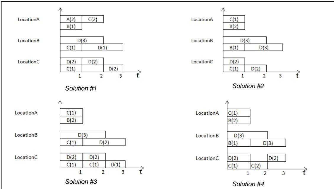
Figure 5: Four best evacuation route plans for the example. Y-axis represents departing locations, X-axis evacuation time, and rectangles route scheduling and the number of evacuees on each route
