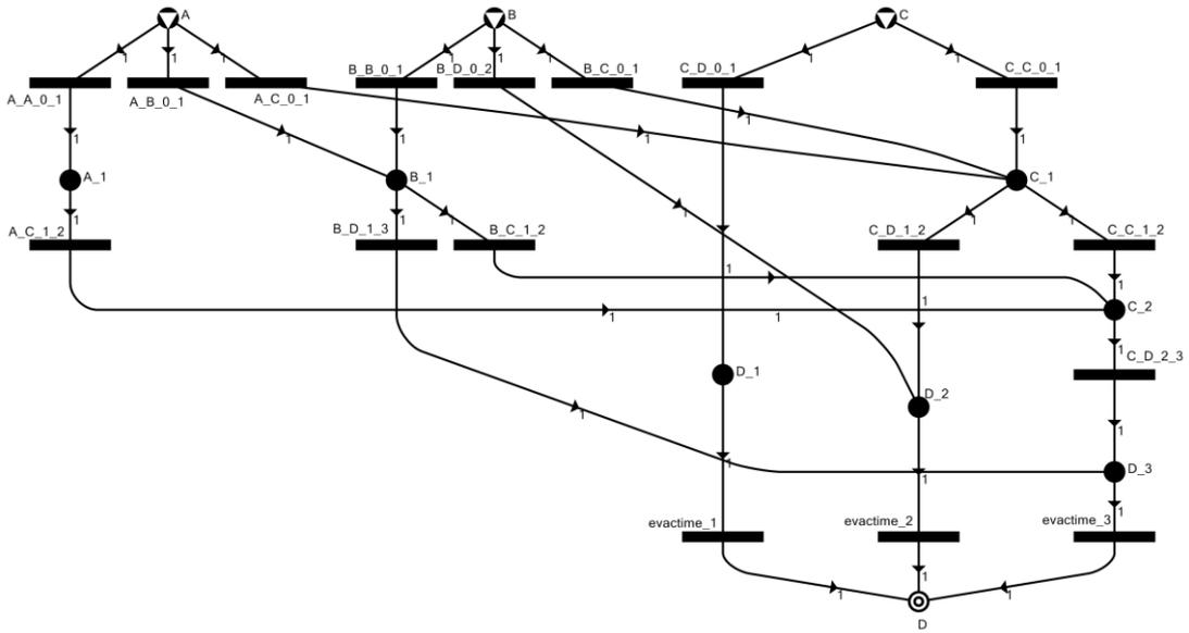
Figure 4: P-graph representation of the maximal structure for Figure 2 (Upper bound of the evacuation time  $T = 3$ )
