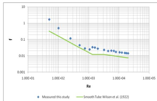
Figure 3 Comparison of the measured / reduced friction factor data versus Reynolds number for the Vipertex 1EHT and a smooth tube, in an inside fluid cooling arrangement.
