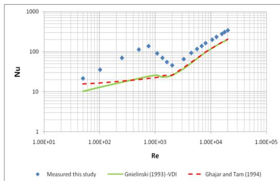
Figure 2 Comparison of the measured / reduced Nusselt number data versus Reynolds number for the Vipertex 1EHT and a smooth tube, in an inside fluid cooling arrangement.
