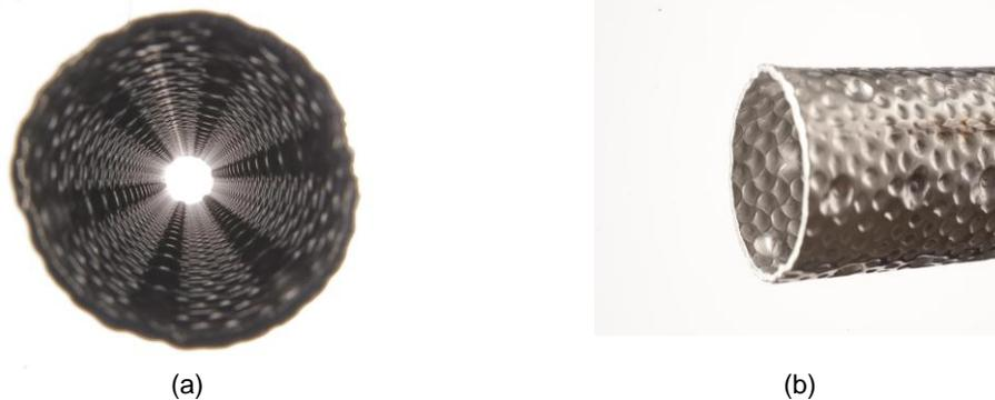
*Figure 1: Photographs of the Vipertex 1EHT tube evaluated in this study (a) Interior Cross Section (b) Detailed Outside Surface*
