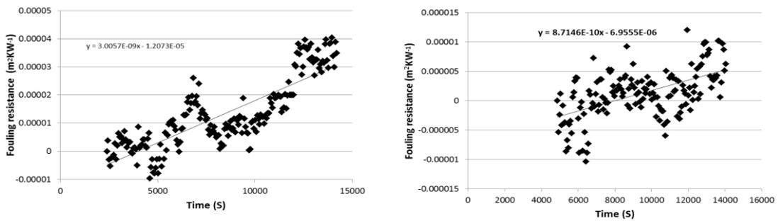
Figure 2 Fouling resistance curves
