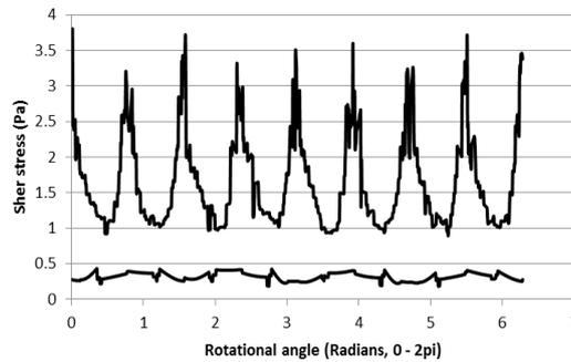
Figure 4 Shear stress distribution around the probe surface at the mid vertical position (0.04 m) in respect of the rotational angle from zero to  $2\pi$
