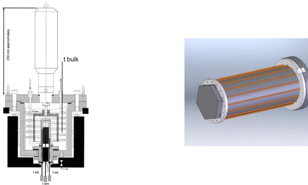
Figure 1 Left: The stirred cell system (Young et al., 2011); *twb*, *twm*, and *tws* are thermocouples Right: modified probe with wire nest on surface, the “wired probe” (for illustration only)
