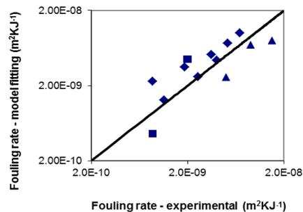
Figure 7. Comparison of the experimental data and the model predictions for the fouling rate
