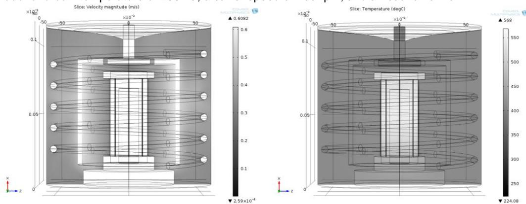
Figure 3 Velocity and temperature fields for the fluid flow in the stirred cell fitted with the wired probe
