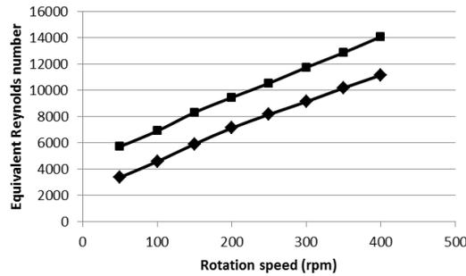
Figure 6. Equivalent Reynolds number for the crude fluid flow in the stirred cell
