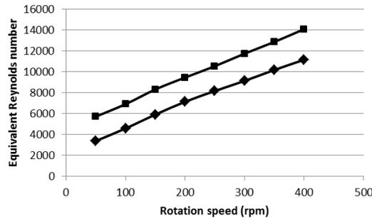
Figure 6. Equivalent Reynolds number for the crude fluid flow in the stirred cell
