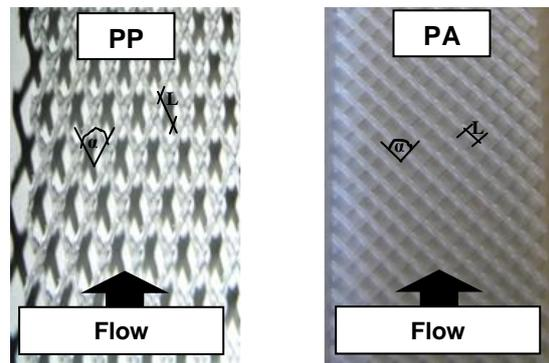
Figure 3: Experimentally investigated spacer geometries.
