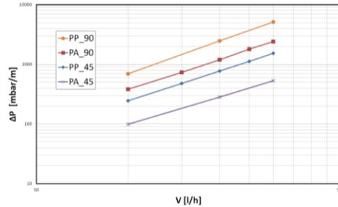
Figure 9: Pressure drop as a function of flow rate at different spacer angles.
