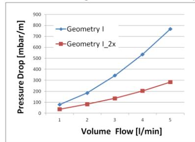
Figure 11: Pressure drop as a function of flow rate for different geometries.
