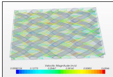
Figure 12: Visualisation of turbulent flow pattern within an interwoven spacer grid
