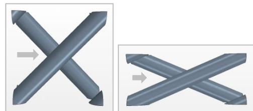
Figure 8: Change in spacer angle for PA grid geometry.
