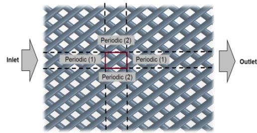
Figure 5: Selection of a periodic element with the respective boundary conditions.
