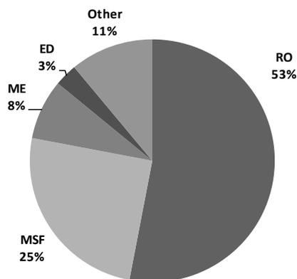
Figure 2: Global desalination capacity by process (ESCWA, 2009)
