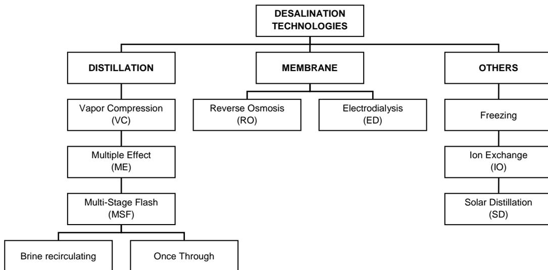
Figure 1: Classification of desalinating processes
