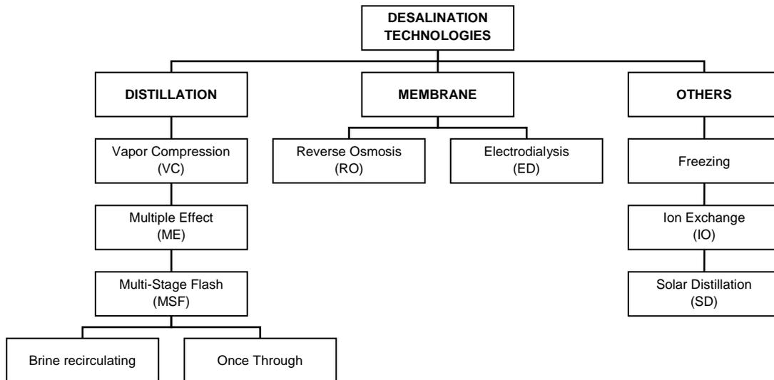
Figure 1: Classification of desalinating processes
