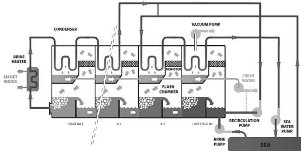
Figure 4: Flow diagram of a new desalination unit
