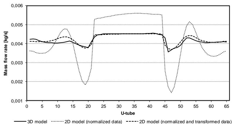
Figure 4: Comparison of flow rates through the middle row of U-tubes (3D model) and through tubes in the simplified 2D model. The transformation used here is  $0.2 \cdot X + 0.0034$  with  $X$  denoting a normalized 2D flow rate.
