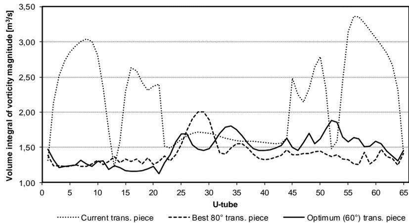
Figure 7: Comparison of volume integrals of vorticity magnitude over inlet parts of individual U-tubes (2D models)
