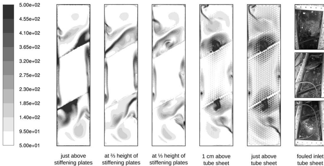
Figure 3: Vorticity magnitude (1/s) in cuts above the inlet tube sheet (3D model); the pattern above closely resembles deposition of particles in the existing preheater depicted right
