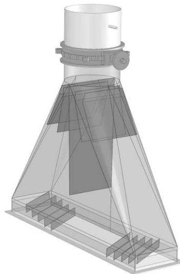
Figure 10: 3D sketch of the optimum inlet transition piece with darkened key parts: throttle valve (top) and guiding vanes (middle and bottom)
