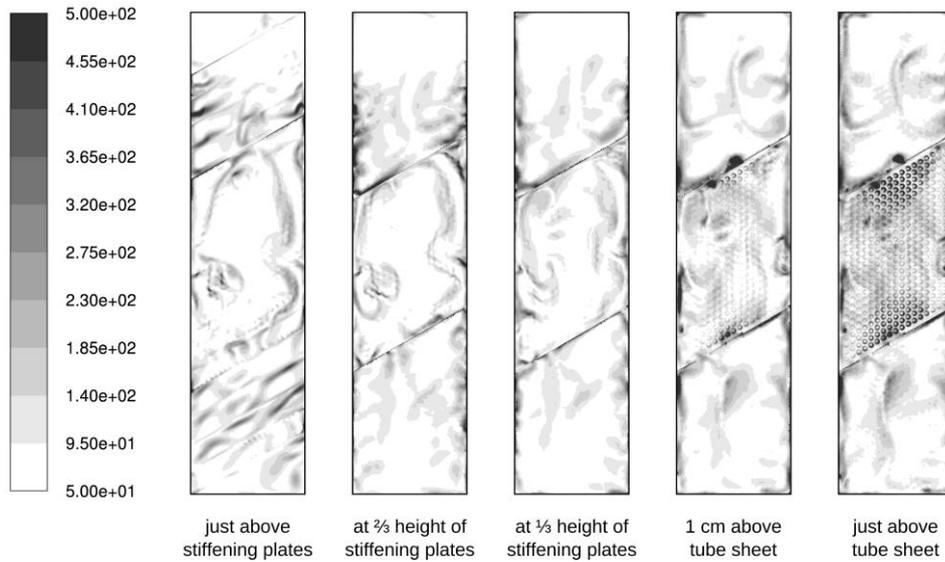
Figure 9: Vorticity magnitude (1/s) above inlet tube sheet in the optimum inlet region geometry
