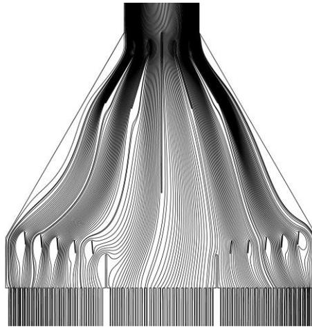
Figure 5: Pathlines in a simplified 2D model of the optimum inlet region
