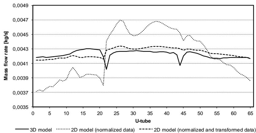
Figure 8: Comparison flow rates obtained using 2D and 3D models; the transformation used here is the same as the one employed in Figure 4
