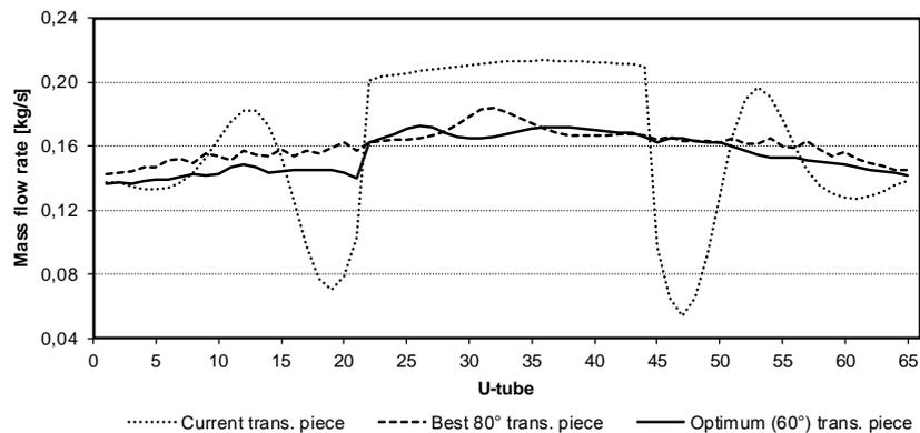
Figure 6: Comparison of flow rates obtained with simplified 2D models
