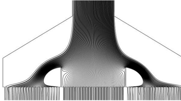
Figure 2: Pathlines in a simplified 2D model of the existing inlet region; empty areas are stagnation zones
