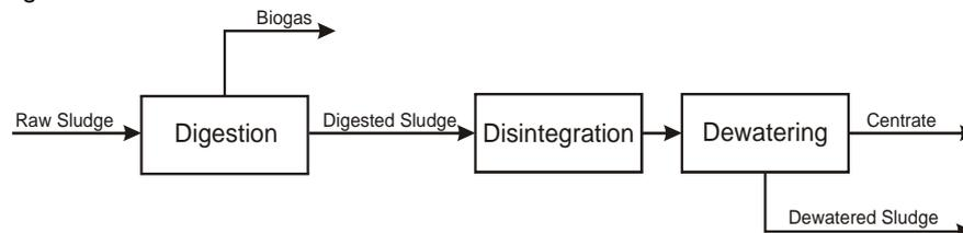
Figure 1: Flow diagram of sludge management for enhanced dewatering
