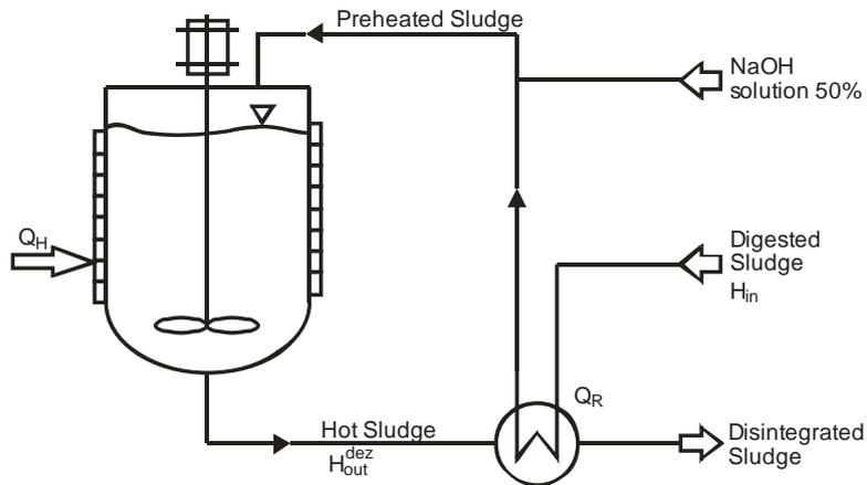
Figure 2: Flow diagram of disintegration process
