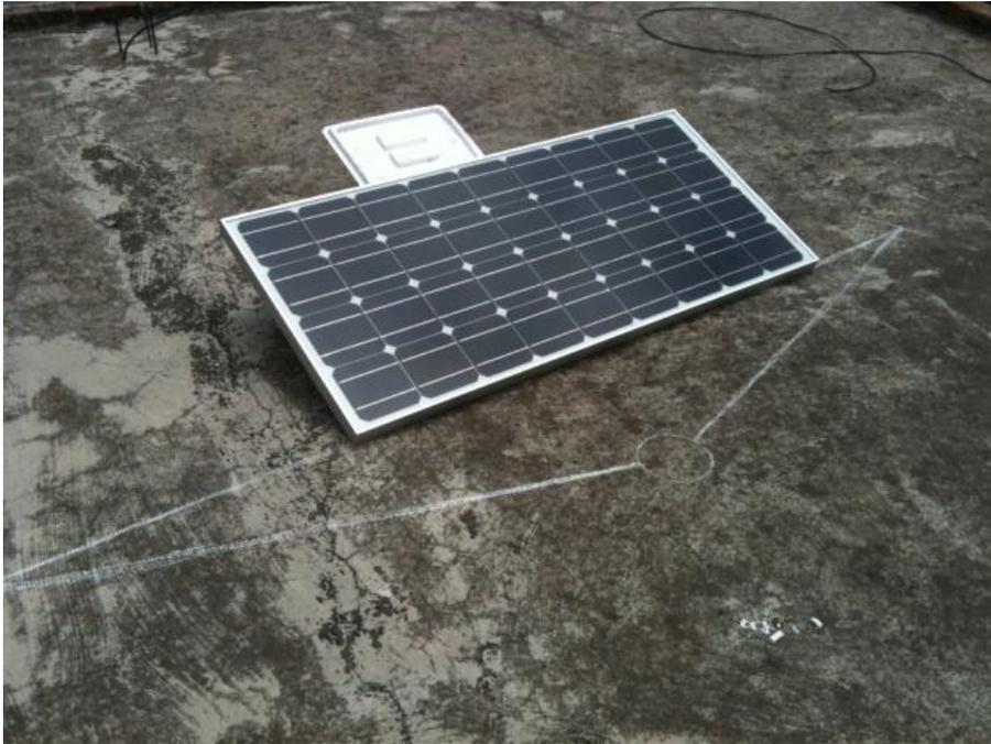
Figure 3: Mono-crystalline Solar Panel.
