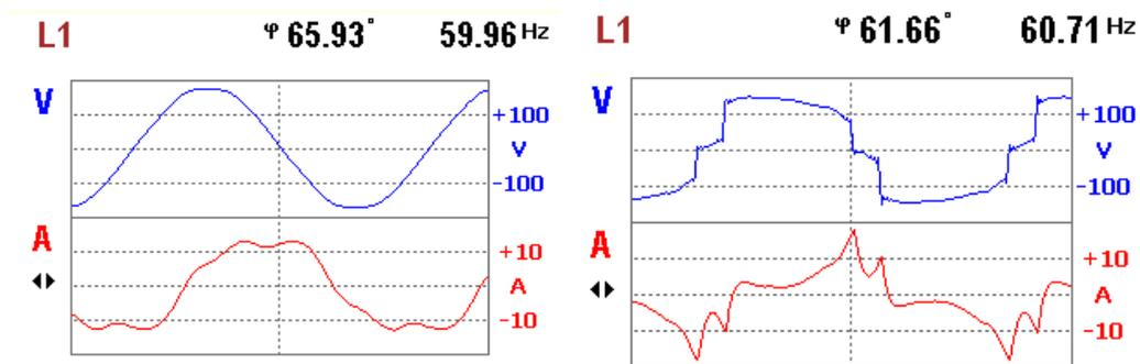
a) Electrical Grid b) PV system (Inverter)
