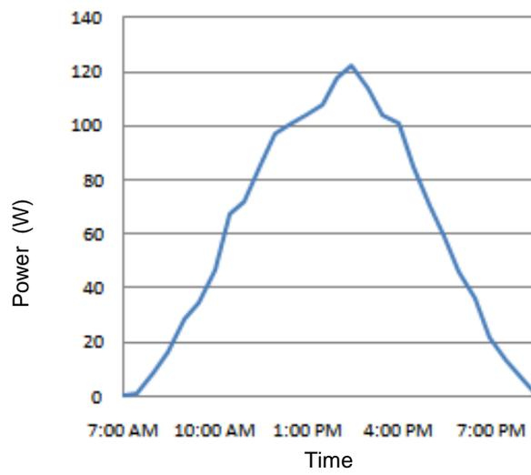
Figure 4: Power Generation Curve of PV system.
