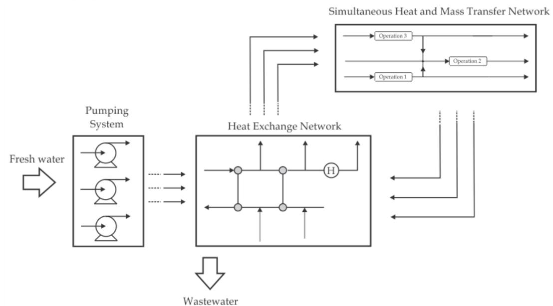
Figure 1. Power, mass and heat integration system (PMHI)
