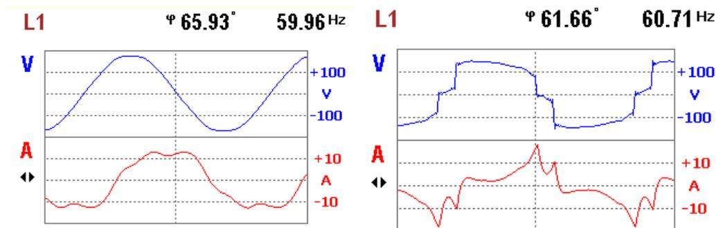
a) Electrical Grid b) PV system (Inverter)
