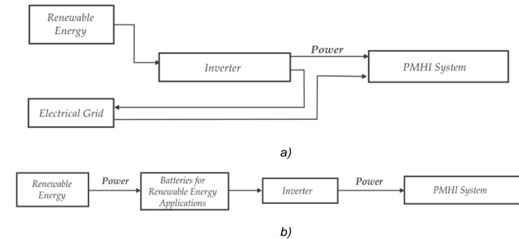
Figure 2. a) Power generated by renewable energy along with supply from the electric grid; b) power is generated by renewable energy and a set of batteries supply the power to the PMHI system.
