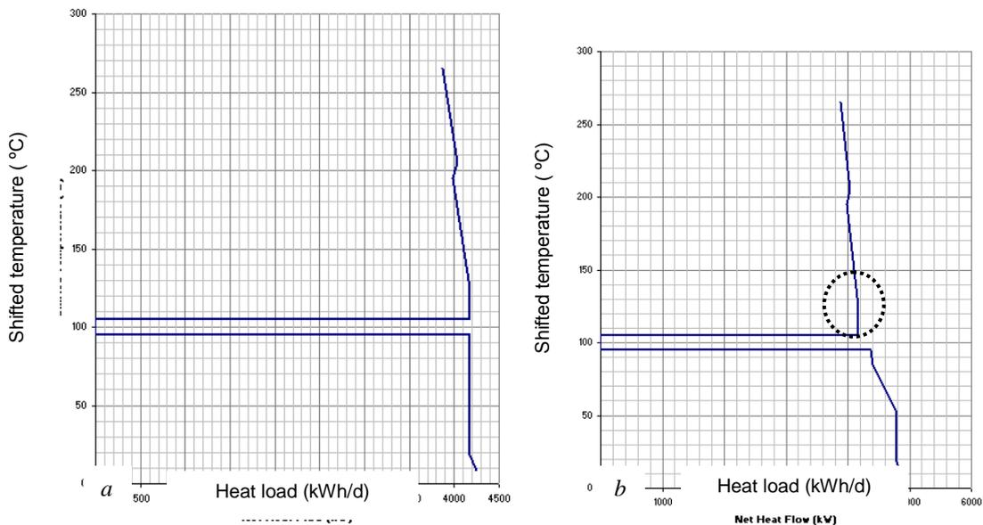
Figure 2: GCC of Scenarios before incorporating thermosolar energy; a. Scenario 1, and b. Scenario 2
