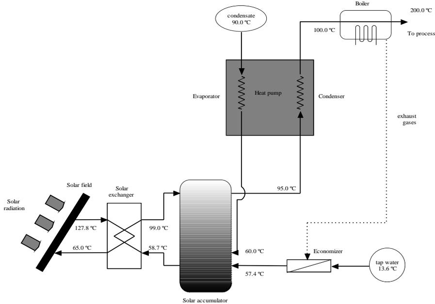
Figure 3: energy supplying system for Scenario 3
