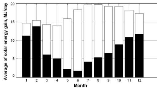
Figure 2. Average solar energy gain (black) bar and the total energy required for the household to heat water (white bar) for month
