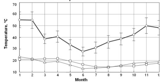
Figure 1. Output temperature of the system at noon. The circles represent the output temperature, squares: the water of the network (average for month); triangles: ambient temperature.
