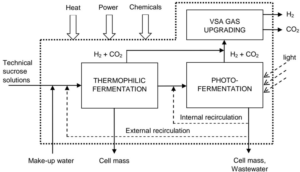
Figure 1: Block diagram of the two-stage fermentative processing of sucrose to hydrogen
