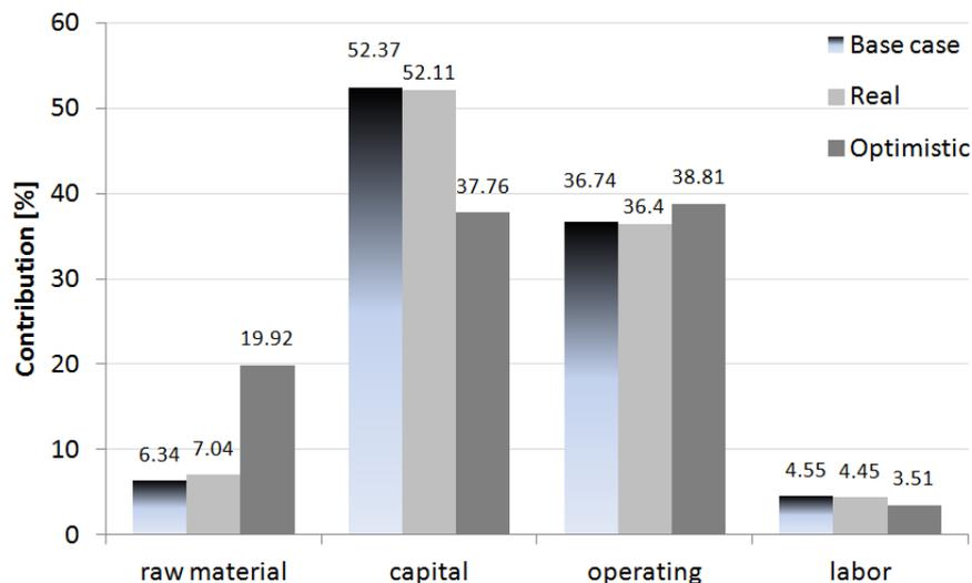
Figure 2: H<sub>2</sub> production cost structure
