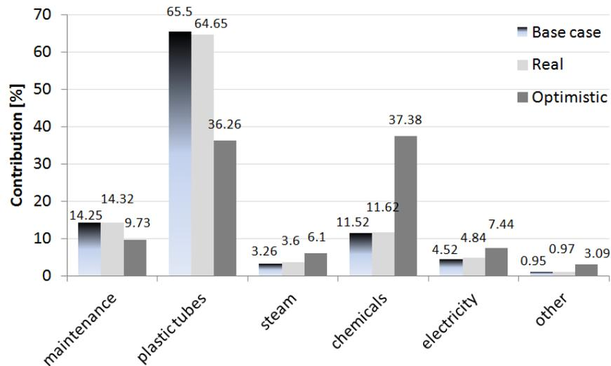
Figure 4: Operating cost structure
