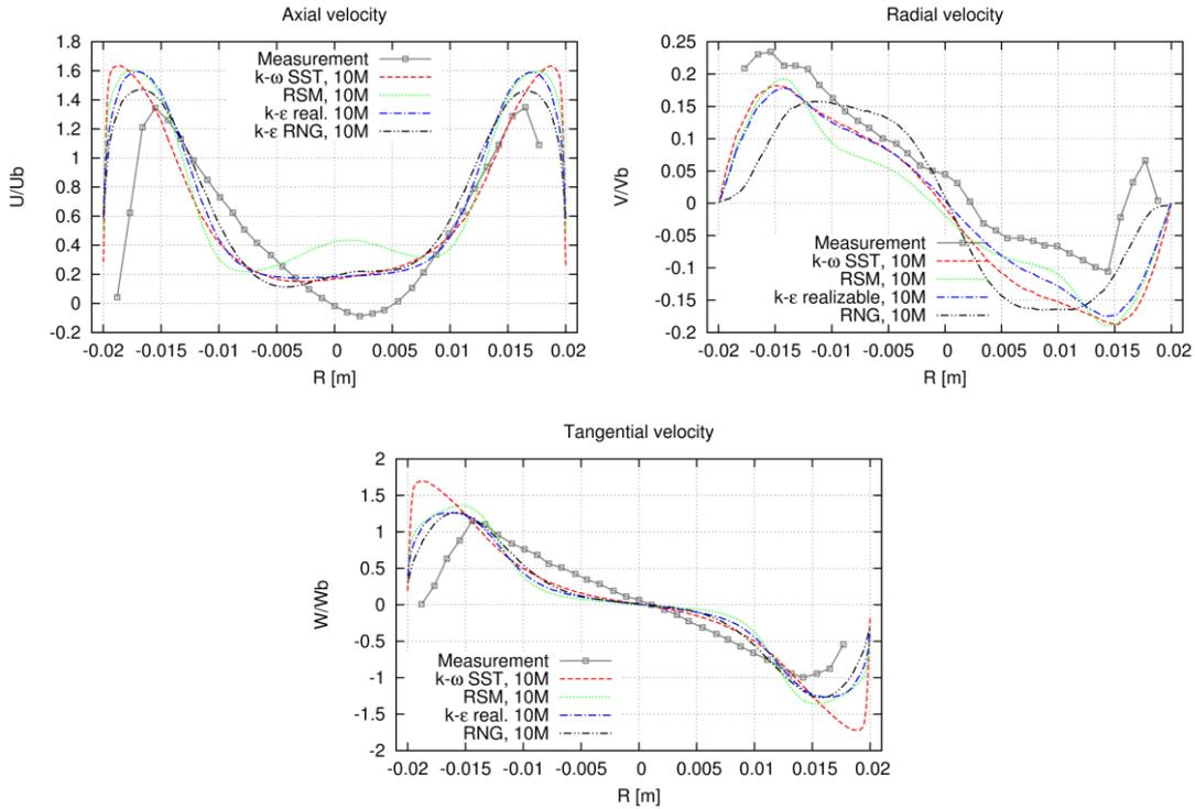
Figure 2: Profiles of axial, radial and tangential velocity in the highest density mesh for four turbulence models
