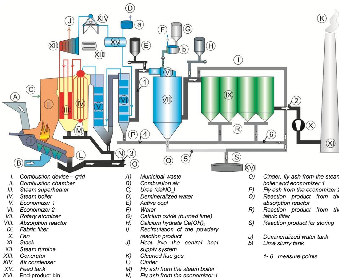
Figure 2: Description of flows a measure points in the incineration plant
