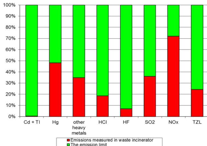
Figure 5: Comparison of concentrations of pollutants measured in the incineration plant with emission limits valid in the EU (Directive, 2000)
