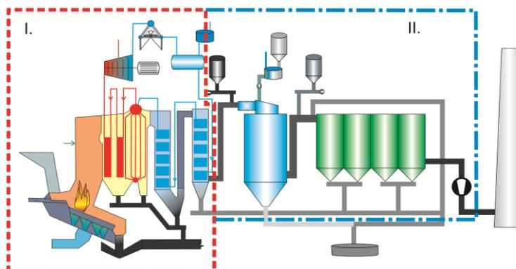
Figure 3: Division of the incineration plant to computation circuits
