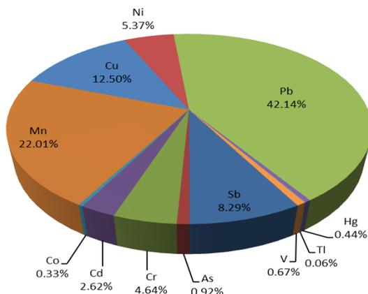
Figure 1: The share of particular elements in the fly ash drifted by flue gas from combustion chamber in the evaluated case
