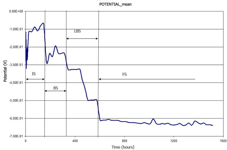
Figure 1: Paint Nº 01 Mean potential variation with time
