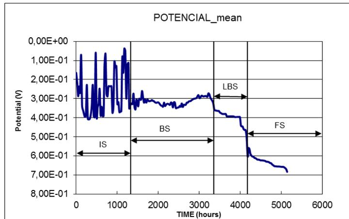
Figure 3: Paint N° 03 Mean potential variation with time
