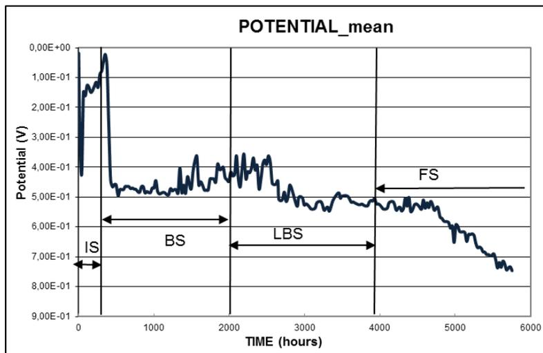
Figure 4: Paint N° 04 Mean potential variation with time
