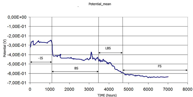
Figure 2: Paint Nº 02 Mean potential variation with time
