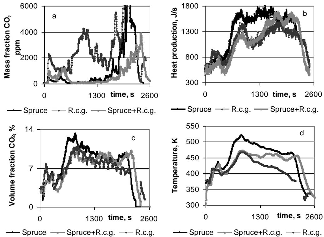
Figure 2: Time-dependent variations of (a) volatiles (CO) formation, (b) rate of heat energy production, (c) main product (CO<sub>2</sub>) formation and (d) product temperature at the thermo-chemical conversion of densified biomass under stoichiometric combustion conditions ( $\alpha \approx 1$ ) downstream the combustor.
