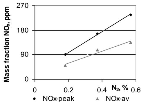
Figure 3: Correlation between the NO<sub>x</sub> emissions and the nitrogen content in biomass samples.
