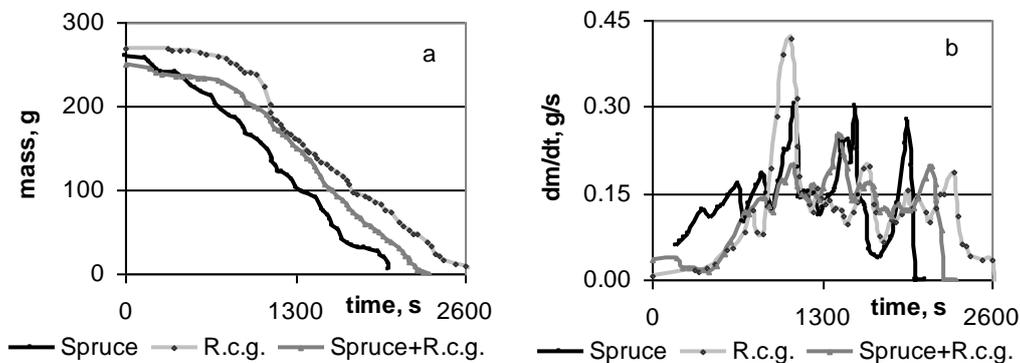
Figure 1: Time dependent variations of the mass loss (a) and mass loss rates (b) for different types of densified biofuels at the primary air supply rate 0.6 g/s.
